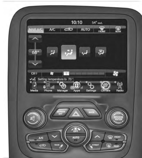
8.4 NAV Temperature Controls
