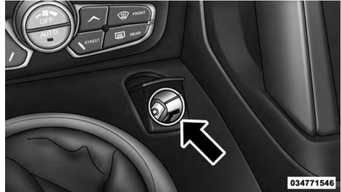
Front Power Outlet
