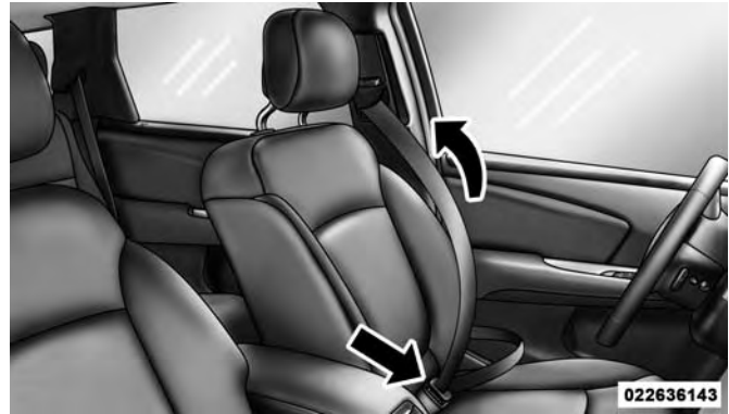
Positioning The Lap Belt
