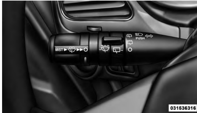
Windshield Wiper/Washer Lever
