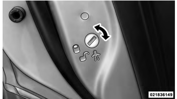
Child-Protection Door Lock Function
