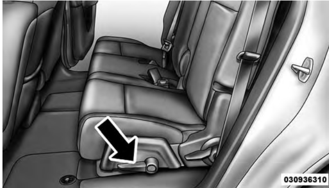
Seat Track Release Lever
