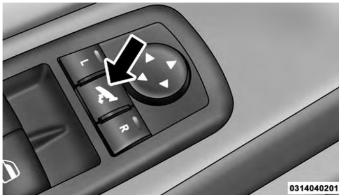
Power Folding Mirror Switch
