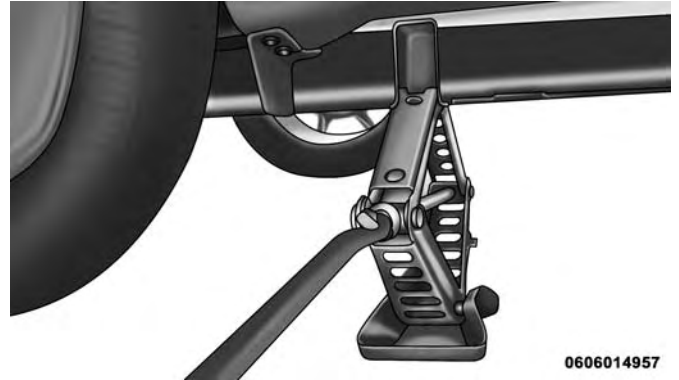
Rear Jack Engaged With Jack Handle
