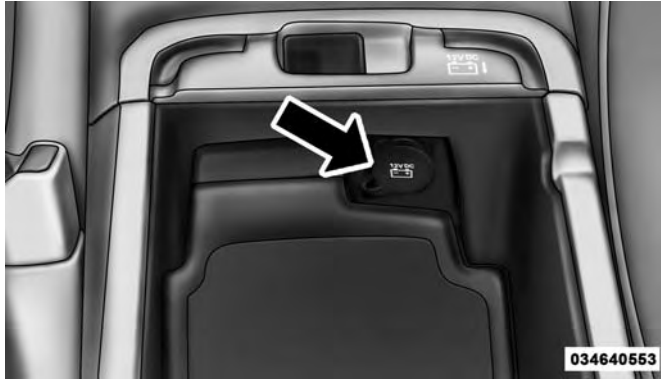
Front Center Console Outlet
