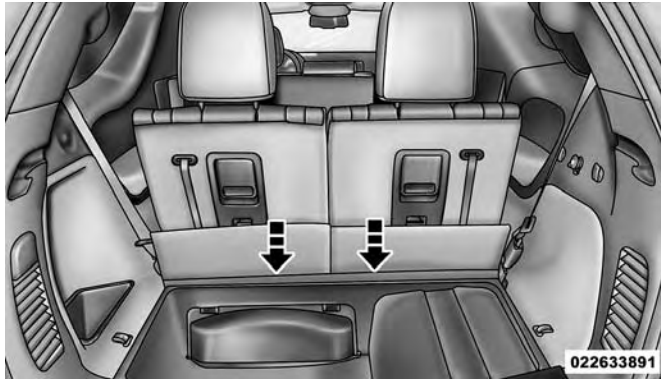
Pulling Down The Carpet Floor Panel To Access Top Tether Strap Anchorage
