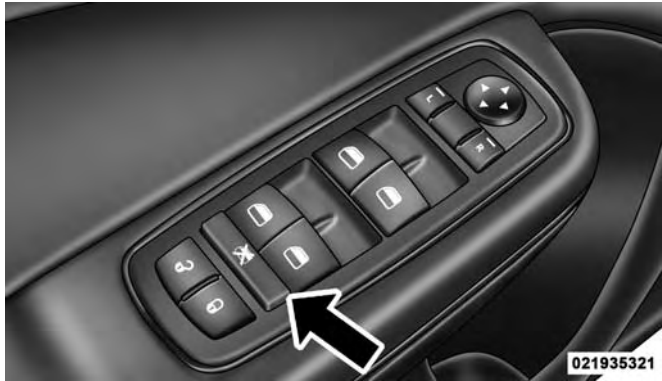
Window Lockout Switch
