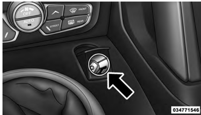
Front Power Outlet
