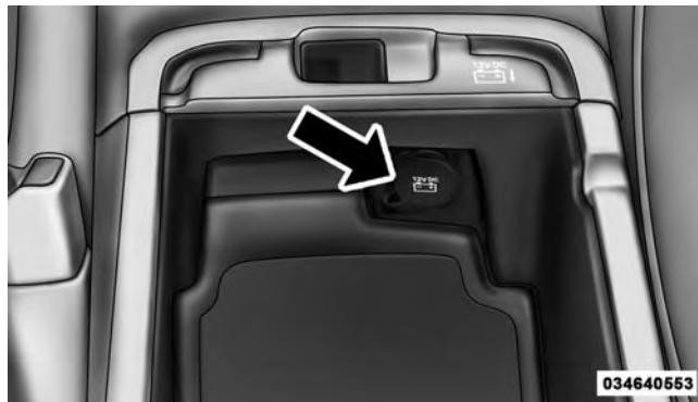
Front Center Console Outlet
