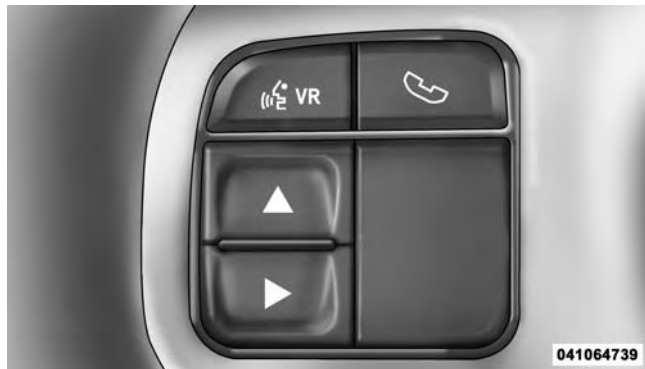
EVIC Steering Wheel Buttons (Two-Button EVIC Controls)
