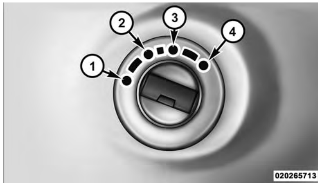
Ignition Node Module (IGNM)
