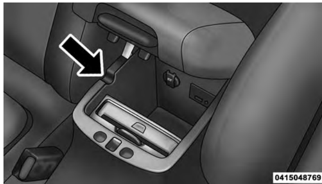
Center Console USB/AUX Connector Port Cable Routing
