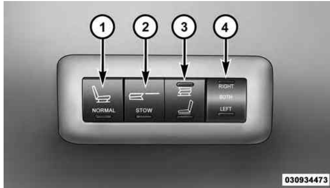
Rear Panel Power Switch Bank
