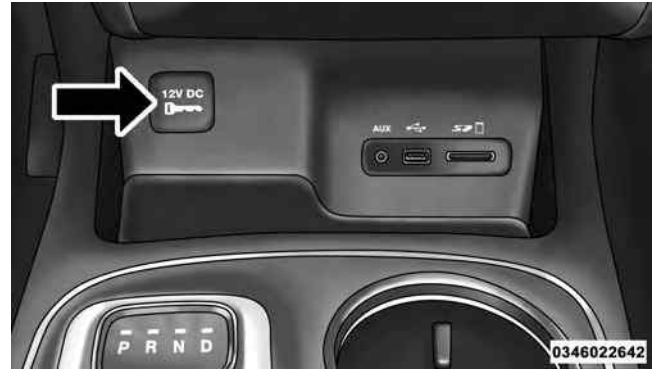
Front Power Outlet
