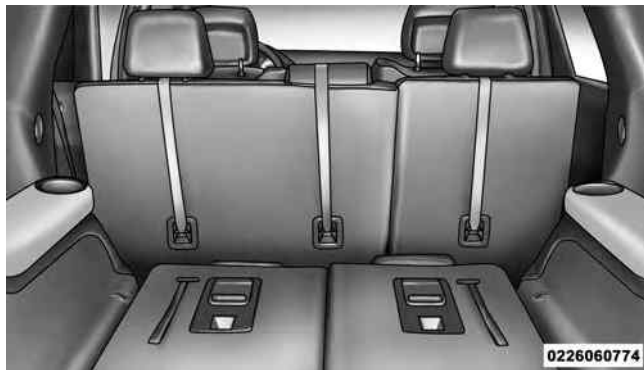
Top Tether Strap Mounting (60/40 Seat)
