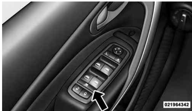
Window Lockout Switch
