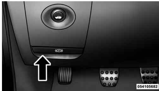
Manual Transmission Parking Brake Release
