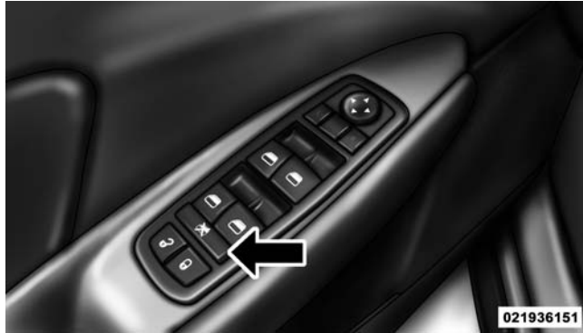
Window Lockout Switch
