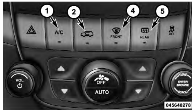
Automatic Temperature Controls — Hard-Keys
