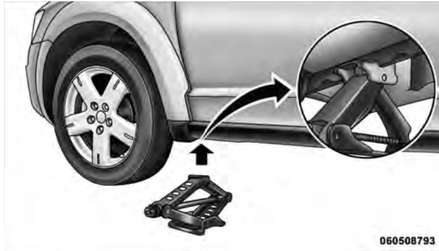
Front Jacking Location
