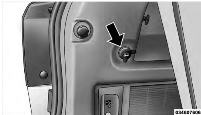
Rear Power Outlet
