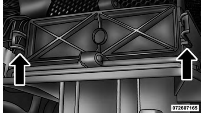
A/C Air Filter Replacement
