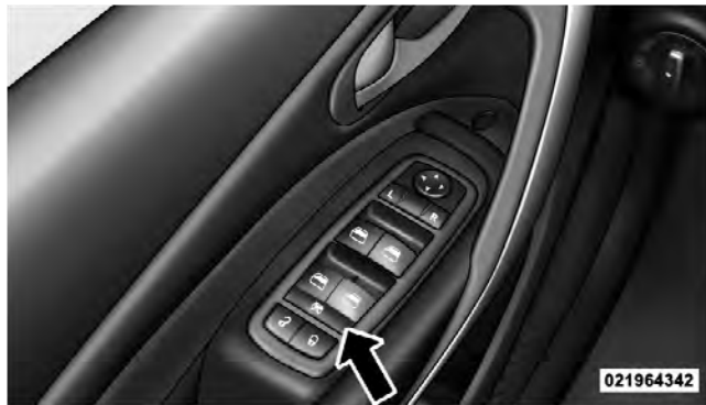
Window Lockout Switch
