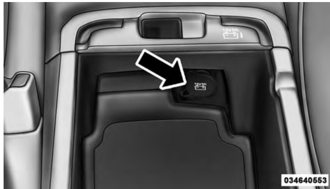
Front Center Console Outlet
