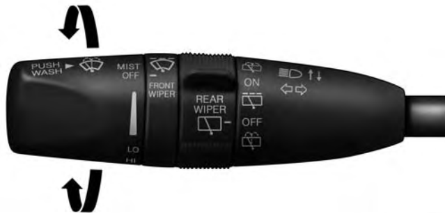
Windshield Wiper Operation
