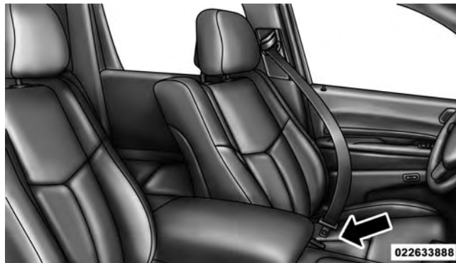
Latch Plate To Buckle
