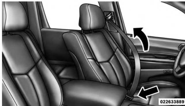
Removing Slack From Belt
