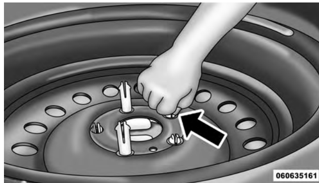
Releasing Protective Plate
