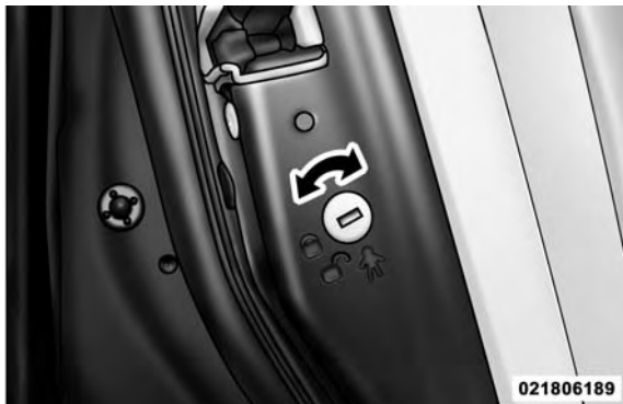
Child-Protection Door Lock Function
