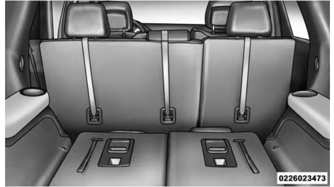
Top Tether Strap Mounting (60/40 Seat)
