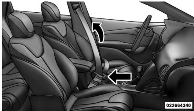
Removing Slack From Belt
