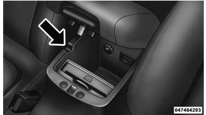
Center Console USB/AUX Connector Port Cable Routing
