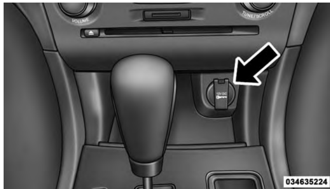
Front Power Outlet
