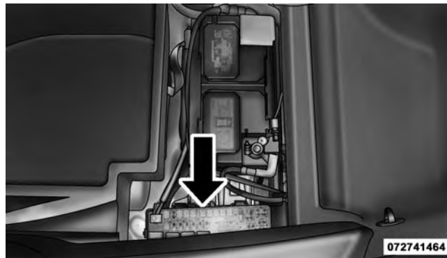
Rear Power Distribution Center
