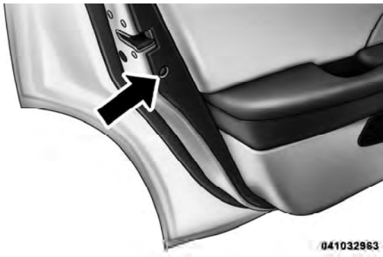
Child-Protection Door Lock Location
