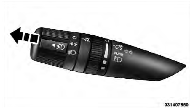
Front Fog Light Control
