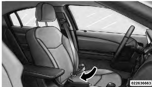
Inserting Latch Plate Into Buckle
