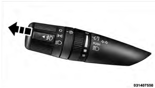
Front Fog Light Control
