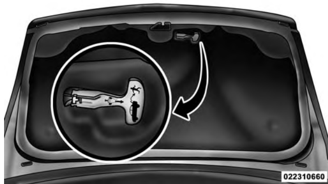
Trunk Internal Emergency Release
