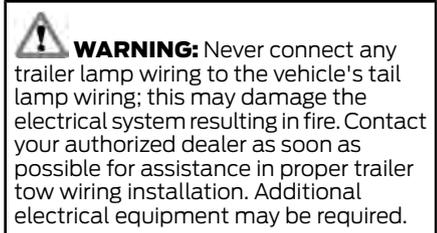
Trailer lamps are required on most towed vehicles. Make sure all running lights, brake lights, direction indicators and hazard lights are working.
