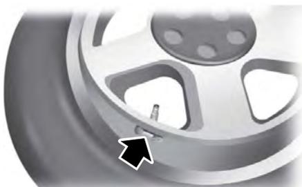
**Note:** *Each road tire is equipped with a tire pressure sensor located inside the wheel and tire assembly cavity. The pressure sensor is attached to the valve stem. The pressure sensor is covered by the tire and is not visible unless the tire is removed. Take care when changing the tire to avoid damaging the sensor.*
