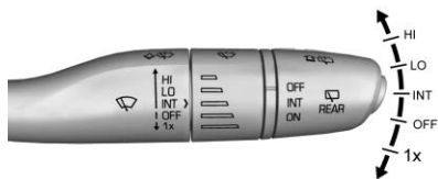
Windshield Wiper without Rainsense (INT Shown)
