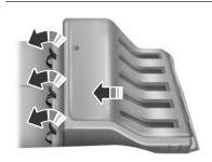
5. Release the three clamps that secure the cover to the air filter housing. Push the air filter cover toward the center of your vehicle, and up slightly, to release it
