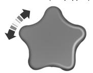
The lumbar support control is located on the outboard side of the seat. Turn the control to adjust your support.
