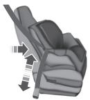
8. Before placing the child into the child seat, forcibly pull the child seat forward and back to make sure that the seat is held securely in place. To check this, grab the seat at the belt path and attempt to move it side to side and forward and back. There should be no more than 1 inch (2.5 centimeters) of movement for proper installation.
