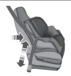
9. Before placing the child in the seat, forcibly move the seat forward and back to make sure the seat is securely held in place.
