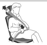
Pregnant women should always wear their safety belts. The lap belt portion of a combination lap and shoulder belt should be positioned low across the hips below the belly and worn as tight as comfort will allow. The shoulder belt should be positioned to cross the middle of the shoulder and the center of the chest.
