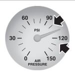
Periodically check the air pressure gauge while driving. Pressure should range between approximately 100–125 psi (690–862 kPa). The air compressor governor cut-in and cutout pressure settings are set at the factory and are not adjustable.
