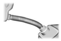
4. Lift and tip the container to let DEF flow into the tank. Pour DEF until the container is empty or DEF flow stops. DEF can be seen flowing through the spout, but does not completely fill the spout while flowing. Air is trapped in the spout while DEF is flowing. When the DEF tank is full, DEF completely fills the spout and displaces the air in the spout.
