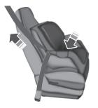
7. Remove remaining slack from the belt. Force the seat down with extra weight (e.g., by pressing down or kneeling on the child restraint while pulling up on the shoulder belt in order to force slack from the belt).
