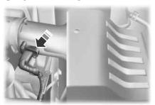
1. Locate and disconnect the mass air flow sensor electrical connector on the air outlet tube.
