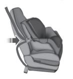
3. While holding both shoulder and lap portions next to the tongue, route the tongue and webbing through the child seat according to the child seat manufacturer's instructions. Be sure that the belt webbing is not twisted.
