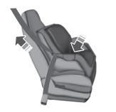
5. While pushing down with your knee on the child seat pull up on the shoulder belt portion to tighten the lap belt portion of the combination lap and shoulder belt.
