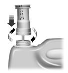
1. Remove the cap from the DEF container and twist the spout onto the container until the locking tab engages.
