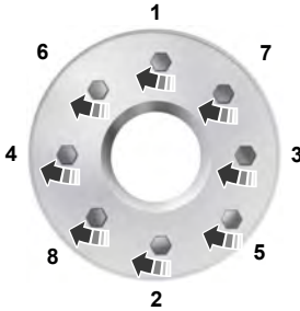
8-lug nut torque sequence
