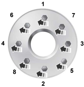
8-lug nut torque sequence
