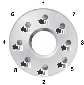
8-lug nut torque sequence
