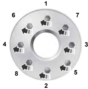
8-lug nut torque sequence
