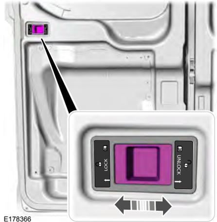
1. Slide the lever to release the catch.
