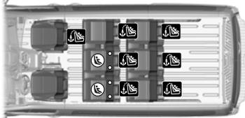
Your vehicle has LATCH lower anchors for child restraint installation at the seating positions marked with the child restraint symbol.
