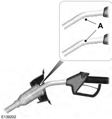
**Note:** When you insert the correct size fuel pump nozzle a spring loaded inhibitor will open.
