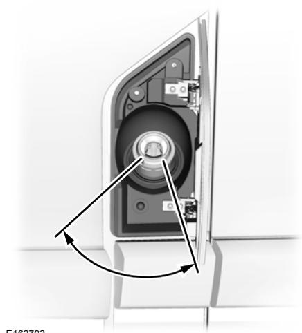
4. Operate the fuel pump nozzle within the area shown.
