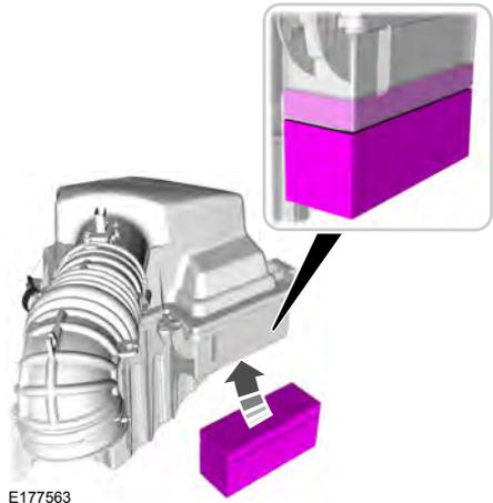
The secondary foam air filter must be in place when the engine is running.
