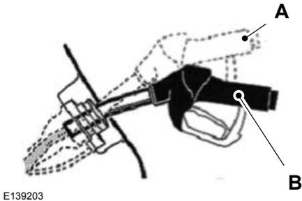
3. Hold the fuel pump nozzle in position B when refueling. Holding the fuel pump nozzle in position A may affect the flow of fuel and shut off the fuel pump nozzle before the fuel tank is full.
