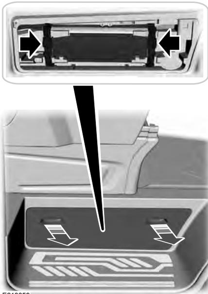
The vehicle jack is under the passenger seat. The jack handle and lug wrench are located in a storage compartment in the front right-hand side stepwell.
