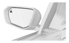
The warning light in the exterior mirror warns of a possible collision with a detected vehicle.
