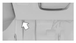
On the driver's side, there is a diagnostic socket for reading out vehicle data.
