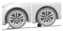
Place wheel chocks or other suitable objects, e.g., rocks, under the wheels of the front axle and rear axle, opposite the rolling direction.
