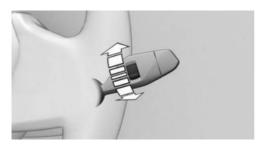
Turn the thumbwheel on the wiper lever.
