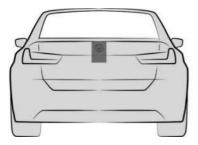
The Rear View Camera is located in the handle strip on the rear of the vehicle.
