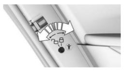
Unlock or lock the safety switch on the rear doors using the integrated key.
