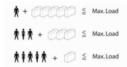
The maximum payload is the sum of the weight of the occupants and the cargo.
