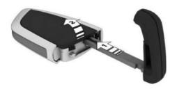
3. Push battery in arrow direction using a pointed object and lift it out.
