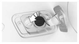
3. Place the fuel filler cap in the bracket on the fuel filler flap.
