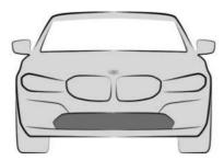
The front radar sensor is located in the front bumper.
