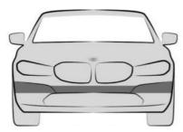
The ultrasonic sensors are located in the front bumper.
