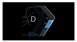
A blue range appears on the power gauge, indicating reduced consumption while driving. If the blue range turns gray, the fuel consumption has increased.
