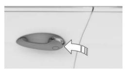
Guide one finger of your other hand from the back under the cover cap and push the cover cap out. Use the thumb for counter support to prevent the cover cap from falling out of the door handle.
