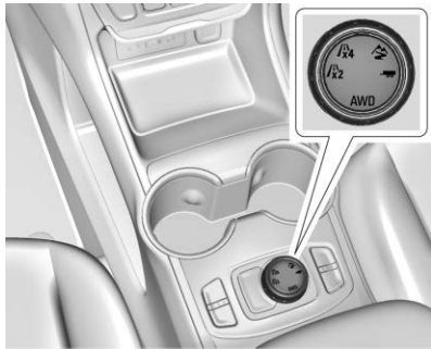
Driver Mode Control Knob for All-Wheel Drive (AWD)
