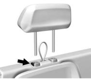
2. Press the button for the passenger side headrest at the top of the seatback and pull up.
