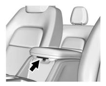
There is storage under the armrest in the center console. Press the button and lift. Depending on the options, there may be a USB port and/or auxiliary jack inside.
