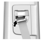
Push up on the release button and move the height adjuster to the desired position.
