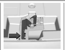
2. Go to the front of the vehicle to find the secondary hood release handle. The handle is under the front edge of the hood near the center. Push the handle to the right and at the same time raise the hood. To close the hood:
