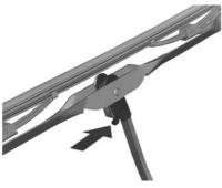
2. Press the release lever in the middle of the wiper blade where the wiper blade attaches.
