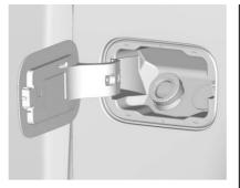
The hinged fuel door is on the driver side of the vehicle. To open the fuel door, push and release the rearward center edge of the door.
