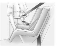
8. Pull the shoulder belt all the way out of the retractor to set the lock. When the retractor lock is set, the belt can be tightened but not pulled out of the retractor.
