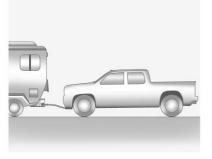
Only dinghy tow four-wheel-drive vehicles that have an N (Neutral) and a Four-Wheel Drive Low (4  $(\downarrow)$  setting.
