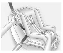
9. To tighten the belt, push down on the child restraint, pull the shoulder portion of the belt to tighten the lap portion of the belt, and feed the shoulder belt back into the retractor. When installing a forward-facing child restraint, it may be helpful to use your knee to push down on the child restraint as you tighten the belt.
