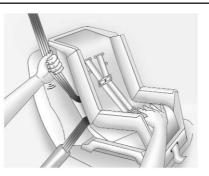
7. To tighten the belt, push down on the child restraint, pull the shoulder portion of the belt to tighten the lap portion of the belt, and feed the shoulder belt back into the retractor. When installing a forward-facing child restraint, it may be helpful to use your knee to push down on the child restraint as you tighten the belt.
