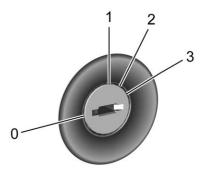
The ignition switch has four different positions.
