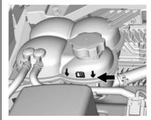
Check to see if coolant is visible in the coolant surge tank. If the coolant inside the coolant surge tank is boiling, do not do anything else until it cools down.
