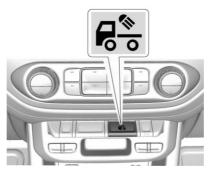
The cargo lamp provides more light in the cargo area of the vehicle, if needed. The lights inside of the pickup box also turn on, if equipped.
