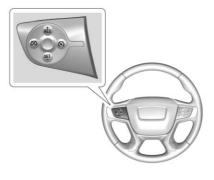
N: Press to turn the system on or off. A white indicator comes on in the instrument cluster when cruise control is turned on.
