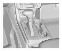
**P** : This position locks the drive wheels. Use P (Park) when starting the engine because the vehicle cannot move easily. When parked on a hill, especially when the vehicle has a heavy load, you might notice an increase in the effort to shift out of P (Park). See "Torque Lock" under *Shifting Into Park* ⇔ 222.
