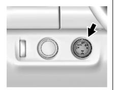
Use the transfer case knob next to the steering wheel to shift into and out of four-wheel drive.
