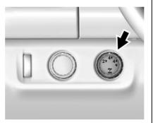
Use the transfer case knob, next to the steering wheel, to shift into and out of four-wheel drive for extra traction. All of the lights will blink on then off momentarily when the ignition is turned on. The light that remains on will indicate the state of the transfer case.
