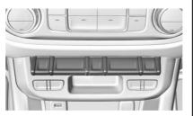
Press this button on the center stack to turn on and off the Tow/ Haul Mode.
