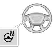
If equipped, press to turn it on or off. A light next to the button displays when the feature is turned on. The steering wheel takes about three minutes to start heating.
