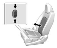
If equipped, press and hold the top of the control to increase lumbar support. Press and hold the bottom of the control to decrease lumbar support. Release the control when the desired level of support is reached.
