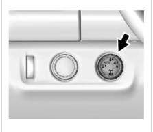
The transfer case knob is to the left of the steering column. Use it to shift into and out of the different four-wheel drive modes.
