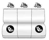
**Crew Cab** Seating positions with top tether anchors. Seating positions with two lower anchors.
