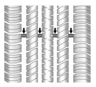
Treadwear indicators are one way to tell when it is time for new tires. Treadwear indicators appear when the tires have only 1.6 mm (1/16 in) or less of tread remaining. Some commercial truck tires may not have treadwear indicators.
