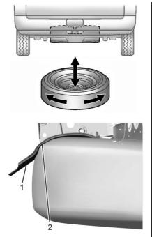
Make sure the tire is stored securely and flush in the radius (2) of the spare tire support bracket (1). Push, pull, and then try to turn the tire. If the tire moves, use the wheel wrench to tighten the cable.
