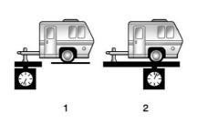
In general, trailer tongue weight (1) should be 10–15% of the loaded trailer weight (2). Some specific trailer types, such as boat trailers, fall outside of this range. Refer to the trailer owner's manual for the recommended trailer tongue weight. In all cases, do not exceed the maximum loads for the vehicle series and hitch type.
