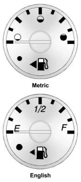
The fuel gauge, when the ignition is on, indicates how much fuel is left in the vehicle fuel tank.
