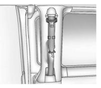
For the second and third row seats, stow the seat belt latch by attaching the clip on the seat belt latch to the trim just inside the side door.
