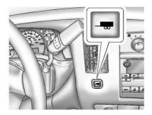
If equipped, Tow/Haul Mode adjusts the transmission shift pattern to reduce shift cycling, providing increased performance, vehicle control, and transmission cooling when towing or hauling heavy loads.
