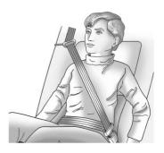
Buckle, position, and release the seat belt as described previously in this section. Make sure that the shoulder belt crosses the shoulder. The belt should be close to, but not contacting, the neck.
