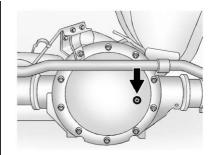
For axles with the fill plug located on the back cover of the rear axle, the proper level is 15 mm to 40 mm (0.59 to 1.57 in) below the bottom of the fill hole.
