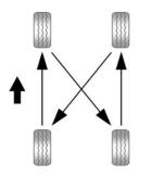
Use this rotation pattern when rotating the tires if the vehicle has single rear wheels.
