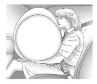
If the vehicle has a front outboard passenger frontal airbag, it is in the passenger side instrument panel.
