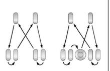
Use this rotation pattern when rotating the tires if the vehicle has dual rear wheels.
