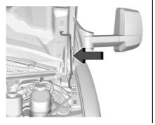
3. Lift the hood, release the hood prop from its retainer, and put the hood prop into the slot in the hood.
