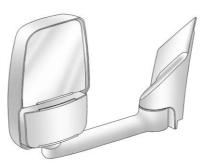
Vehicles with towing mirrors can be adjusted manually for a clear view of the objects behind you.
