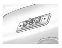
To adjust a power seat, if available, use the controls on the front of the seat:
