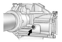
For axles with the fill plug located on the passenger side of the rear axle, the proper level is 0 mm to 10 mm (0 to 0.4 in) below the bottom of the fill hole.
