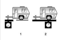
In general, trailer tongue weight (1) should be 10–15% of the total loaded trailer weight (2). Some specific trailer types, such as boat trailers, fall outside of this range. Refer to the trailer owner's manual for the recommended trailer tongue weight. In all cases, do not exceed the maximum loads for the vehicle series and hitch type.
