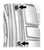
1. Remove the two inboard nuts from the inside of the taillamp assembly.
