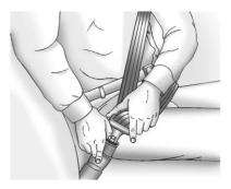
To unlatch the belt, push the button on the buckle. The belt should return to its stowed position. Slide the latch plate up the seat belt webbing when the seat belt is not in use. The latch plate should rest on the stitching on the seat belt, near the guide loop on the side wall.
