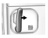
To open the sliding side door from the inside, pull the handle toward the rear of the vehicle. Then, slide the door toward the rear of the vehicle.
