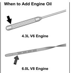
If the oil is below the cross-hatched area at the tip of the dipstick and the engine has been off for at least 15 minutes, add 1 L (1 qt) of the recommended oil and then recheck the level. See "Selecting the Right Engine Oil" later in this section for an explanation of what kind of oil to use. For engine oil crankcase capacity, see *Capacities and Specifications*  $\Rightarrow$  313.
