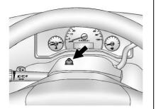
$\triangle$ : Press this button to make the front and rear turn signal lamps flash on and off. This warns others that you are having trouble. Press again to turn the flashers off.
