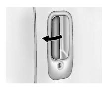
To open the front portion of a 60/40 door from the outside, pull out on the handle and open the door.
