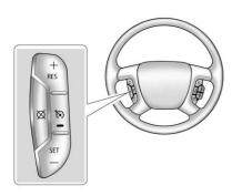
: If equipped, press to turn cruise control on or off. The white indicator comes on in the instrument cluster when cruise control is turned on.
