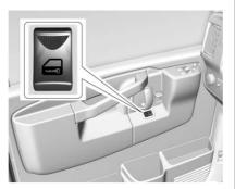
If equipped, press 🖨 to lock or unlock the doors.
