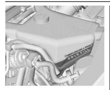
When the engine is cold, the coolant level should be at or above the COLD FILL mark. If it is not, there could be a leak in the cooling system.
