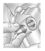
Put the wheel nuts back on with the rounded end of the nuts toward the wheel. Tighten each wheel nut by hand until the wheel is held against the hub. 10. Turn the jack handle counterclockwise to lower the vehicle. Lower the jack completely.
