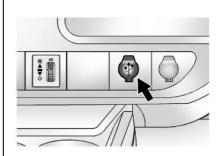
If equipped, the USB port is on the instrument panel and uses the USB 2.0 standard.
