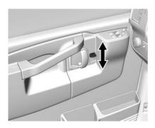
Lock and unlock the door from the outside using the key or the Remote Keyless Entry (RKE) transmitter, if equipped. From the inside, slide the manual lever on the door up or down.
