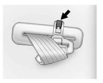
For the last row of seats, stow the seat belt latch plate on the clip at the window trim. Roll the mini-latch into the seat belt webbing and then hook the seat belt latch plate on the clip.
