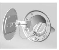
The fuel cap is behind a hinged fuel door on the driver side of the vehicle.
