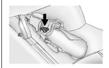
Remove the retaining wing bolt and lift it out of the mounting bracket to access the equipment.
