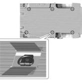
If equipped, there are six cargo tie-downs in the cargo area that can be used to secure cargo.
