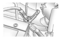
Connect the red positive (+) cable to the positive (+) terminal of the dead battery. Use a remote positive (+) terminal if the vehicle has one. Do not let the other end touch metal. Connect it to the positive (+) terminal of the good battery. Use a remote positive (+) terminal if the vehicle has one.
