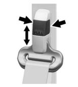
Squeeze both sides of the release button and pull outward. Then move the height adjuster up or down to the desired position and release the button.
