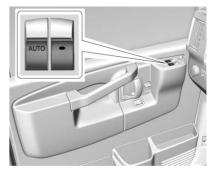
If equipped, power windows work when the ignition is on, in ACC/ ACCESSORY, or when Retained Accessory Power (RAP) is active. See *Retained Accessory Power* (*RAP*) ⇔ 175.
