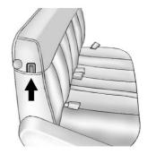
1. Locate the guide in a pocket on the side of the seatback.
