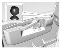
If equipped with power mirrors, select each mirror by turning the knob clockwise for the passenger side mirror or counterclockwise for the driver side mirror. Adjust the mirror angle by moving the knob in the desired direction.
