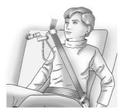
Adjustable comfort guides are available through your dealer for the left rear outboard seating positions of the three-passenger bench seats and for the outboard seating positions of the four-passenger bench seats. Instructions are included with the guides.
