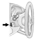
For vehicles with a tilt steering wheel, the lever is located on the left side of the steering column.
