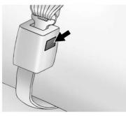
To do this, press the tip of a key into the release hole of the seat belt buckle while pulling up on the seat belt. 2. Locate the pins.
