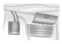
To set the parking brake, hold the regular brake pedal, then push down the parking brake pedal.
