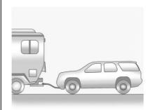
Only dinghy tow four-wheel-drive vehicles with a two speed transfer case that have a N (Neutral) and a 4  $\downarrow$  setting.
