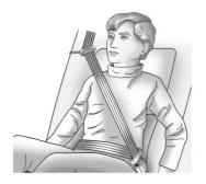
Buckle, position, and release the safety belt as described previously in this section. Make sure the shoulder portion of the belt is on the shoulder and not falling off of it. The belt should be close to, but not contacting, the neck. To remove and store the comfort guide, squeeze the belt edges together so that the safety belt can be removed from the guide. Slide the guide onto its storage clip.
