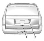
To open the liftgate, press a on the power door lock switch or press a on the RKE transmitter twice to unlock all doors. Press the touch pad (1) on the underside of the liftgate handle and lift up.
