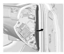
The right instrument panel fuse block access door is on the passenger side edge of the instrument panel.
