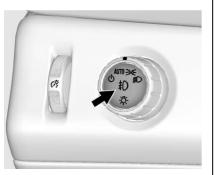
If equipped with fog lamps, the button is on the exterior lamp control, to the left of the steering column.
