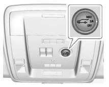
If equipped, the switch is on the overhead console. The vehicle must be in P (Park).
