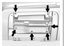
3. Remove the six screws and remove the access plate.
