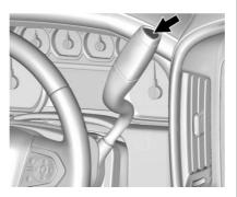
Pressing this button at the end of the shift lever turns on and off the Tow/Haul Mode.
