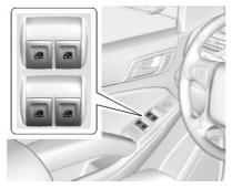
The windows work when the vehicle is in ON/RUN, ACC/ACCESSORY, or when Retained Accessory Power (RAP) is active. See *Retained Accessory Power* (*RAP*) ⇔ 223.
