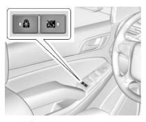
Press at to activate the safety locks on the rear doors. The indicator light comes on when activated.
