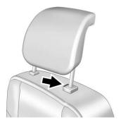
The third row seat head restraint can be lowered to allow for better visibility when the rear seat is unoccupied. To lower the head restraint, press the button located on the top of the seatback and push the head restraint down.
