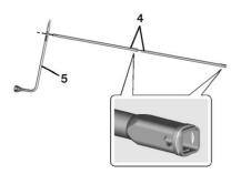
Assemble the two jack handle extensions (4) and wheel wrench (5).
