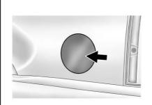
To open the fuel door, push and release the rearward center edge of the door.
