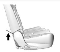
2. Pull the strap on the bottom rear of the second row seat to release the seatback. The seatback will fold forward.
