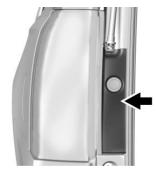
2. Remove the taillamp closeout cover from the lamp assembly by pulling rearward from the top and bottom at the same time to unfasten the snap tabs.
