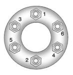
11. Tighten the nuts firmly in a crisscross sequence as shown by turning the wheel wrench clockwise.
