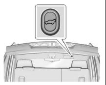
Press any liftgate button, the touch pad, or  $\frac{1}{42}$  on the RKE transmitter while the liftgate is moving to stop it. Pressing any liftgate button or pressing  $\frac{1}{42}$  twice quickly on the RKE transmitter restarts the operation in the reverse direction. Pressing the touch pad on the liftgate handle will restart the motion, but only in the opening direction.
