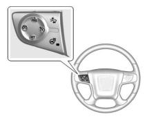
$\ensuremath{\mathfrak{S}}$  : Press to turn the system on or off. A white indicator comes on in the instrument cluster when the cruise is turned on.
