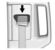
Push down on the release button to move the height adjuster to the desired position.
