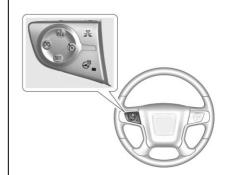
N: Press to turn the system on or off. The indicator turns white on the instrument cluster when ACC is turned on.
