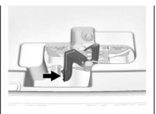
2. Go to the front of the vehicle to find the secondary hood release. The handle is under the front edge of the hood near the center. Push the handle to the right and at the same time raise the hood. Before closing the hood, be sure all the filler caps are on properly. Then bring the hood from full open to within 15 cm (6 in) from the closed position, pause, and push the front center of the hood with a swift, firm motion to fully close the hood.
