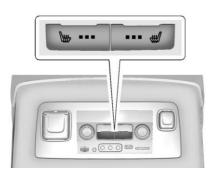
The buttons are on the rear of the center console.
