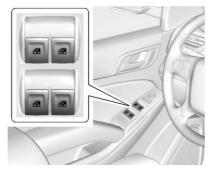
The windows work when the vehicle is in ON/RUN, ACC/ACCESSORY, or when Retained Accessory Power (RAP) is active. See *Retained Accessory Power* (*RAP*) ⇔ 223.
