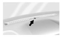
The solar sensor monitors the solar heat. Do not cover the solar sensor or the system will not work properly.
