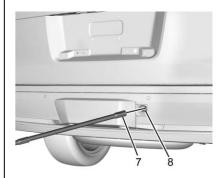
Insert the open end of the extension (7) through the hole in the rear bumper (8) (hoist shaft access hole).
