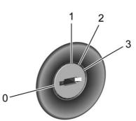
Vehicles with Key Access have an ignition switch with four different positions.
