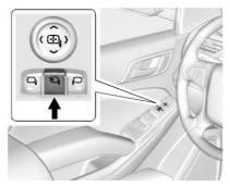
To adjust power folding mirrors, if equipped:
