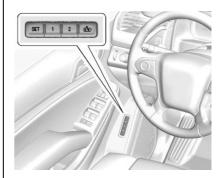
The SET, 1, 2, and 1 (Exit) buttons on the driver door are used to manually store and recall memory settings for the driver seat, outside mirrors, power tilt and telescoping steering column, and adjustable pedals.
