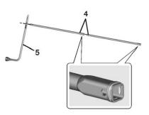
Assemble the two jack handle extensions (4) and wheel wrench (5), as shown.
