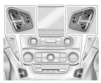
The buttons are on the center stack below the climate control system. To operate, the engine must be running.
