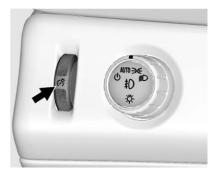
This feature controls the brightness of the instrument panel lights and is next to the exterior lamp control.
