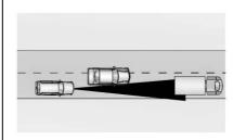
ACC will not detect a vehicle ahead until it is completely in the lane. The brakes may need to be manually applied.
