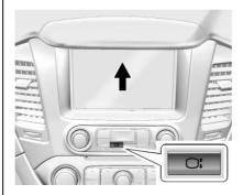
If equipped with storage behind the radio, press and hold  $\bigcirc_{\downarrow}^{\uparrow}$  to open. There is a USB port inside. See the infotainment manual.
