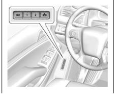
If memory equipped, the SET, 1, 2, and (Exit) buttons on the driver door are used to manually save and recall memory settings for the driver seat, outside mirrors, power tilt and telescoping steering column, and adjustable pedals.
