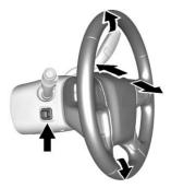
To adjust the power tilt and telescoping steering wheel:
