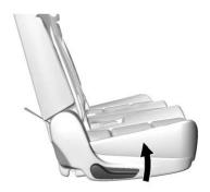
2. Lift the lever, on the outboard side of the seat, to release the seatback.
