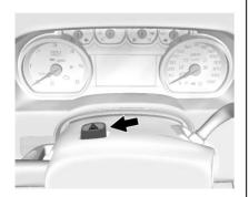
$\triangle$ : Press this button to make the front and rear turn signal lamps flash on and off. Press again to turn the flashers off.
