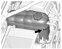
Check to see if coolant is visible in the coolant surge tank. If the coolant inside the coolant surge tank is boiling, wait until it cools down. The coolant level should be at or above the FULL COLD mark. If it is not, there may be a leak in the cooling system.
