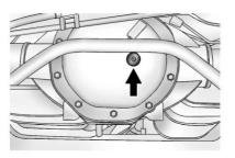
The proper level is 1.0 mm to 19.0 mm (0.04 in to 0.7 in) below the bottom of the fill hole, located on the rear axle. Add only enough fluid to reach the proper level.
