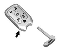
If the vehicle has the Keyless Access system, the transmitter has a button on the side of the transmitter used to remove the key. Do not pull the key out without pressing the button.
