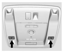
There are reading lamps in the overhead console and the headliner, if equipped. To operate, the ignition must be in the ACC/ACCESSORY or ON/RUN position or using Retained Accessory Power (RAP).
