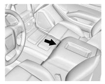
Pull the handle and lift to access. There are auxiliary jacks, USB ports, an accessory power outlet, a tote compartment, and a device holder inside.
