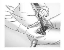
For front seating positions, if the webbing locks in the latch plate before it reaches the buckle, tilt the latch plate flat to unlock.
