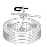
Use the wheel wrench hook to pull the hoist cable closer to assist in reaching the spare tire.
