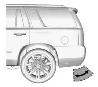
To operate, move your foot in a forward kicking motion under the center of the rear bumper, then pull it back.
