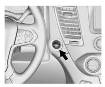
Vehicles with Keyless Access have pushbutton starting.
