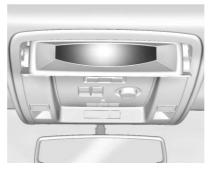
If equipped, push up on the sunglasses bin and release. Push the bin back in halfway to secure the mirror in position.
