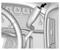
The Tow/Haul Mode adjusts the transmission shift pattern to reduce shift cycling. This provides increased performance, vehicle control, and enhanced transmission and engine cooling when driving down steep hills or mountain grades, towing, or hauling heavy loads. The selector button is on the end of the shift lever. Turn the Tow/Haul Mode on and off by pressing the button. When the Tow/Haul Mode is enabled, a light on the instrument cluster will come on.
