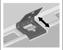
Unsnap the hinges on the load floor from the cargo management system.
