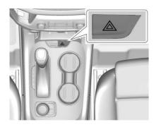
$\triangle$ : Press this button to make the front and rear turn signal lamps flash on and off. This warns others that you are having trouble. Press again to turn the flashers off.
