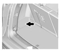
The rear compartment fuse block is behind a trim panel on the driver side of the rear storage compartment.
