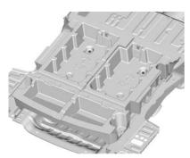
The rear trays do not need to be removed to access the spare tire.
