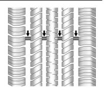
Treadwear indicators are one way to tell when it is time for new tires. Treadwear indicators appear when the tires have only 1.6 mm (1/16 in) or less of tread remaining. See *Tire Inspection*  $\Rightarrow$  327 and *Tire Rotation*  $\Rightarrow$  327.
