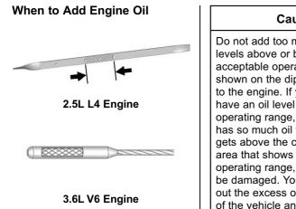
If the oil is below the cross-hatched area at the tip of the dipstick, add 1 L (1 qt) of the recommended oil and then recheck the level. See "Selecting the Right Engine Oil" in this section for an explanation of what kind of oil to use. For engine oil crankcase capacity, see *Capacities and Specifications*  $\Rightarrow$  380.
