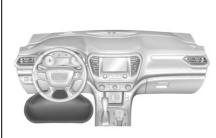
The driver knee airbag is below the steering column.
