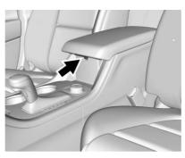
The center console has storage under the armrest. Pull up the latch and lift to open.
