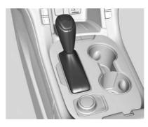
**P**: This position locks the front wheels. It is the best position to use when starting the engine because the vehicle cannot move easily.
