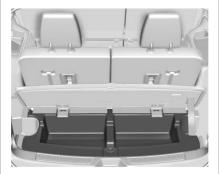
Lift the load floor to access the cargo management system, if equipped with the tray option.
