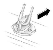
8. Make sure the metal tube is centered at the striker. Push the tube toward the front of the vehicle.
