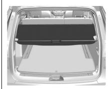
For vehicles with a cargo cover, it can be used to cover items in the rear of the vehicle. Unroll the cover toward the rear of the vehicle. Insert the cover pins into the channels on both sides. To store, carefully remove the cover from the channels and let it roll back up. The cover should be stored securely when not in use.
