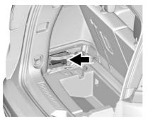
Remove Side Bin, Load Floor and foam. See *Cargo Management System ⇔ 109*
