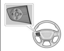
(6): Press to turn the system on and off. A white indicator appears in the instrument cluster when cruise is turned on.
