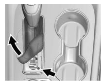
2. Remove the shift lever boot by pulling up on the rear of the trim plate.
