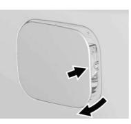
To open the fuel door, push and release the rearward center edge of the door.
