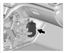
Remove the bolt cap and the screw that attaches the console side trim. Then remove the console side trim to access the fuse block.
