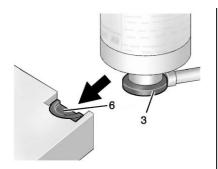
Slide the base of the tire sealant canister (3) into the slot on the top of the compressor (6) to hold it upright.
