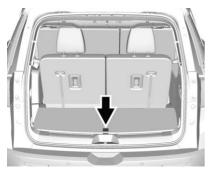
There is storage in the floor of the rear cargo area. Lift the handle to access the removable cargo management system.
