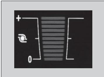
When the turbo charger is producing boost, this meter shows the boost pressure.
