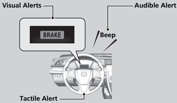
At system's earliest collision alert stage, you can change the distance (**Long/Normal/Short**) between vehicles at which alerts will come on through driver information interface\*/audio/information screen\* setting options.
