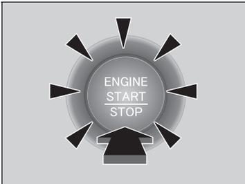
2. Depress the brake pedal (continuously variable transmission) or clutch pedal (manual transmission) and press the **ENGINE START/STOP** button within 10 seconds after the beeper sounds and the **ENGINE START/STOP** button changes from flashing to on.
