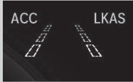
When the LKAS is suspended, the lane lines on the driver information interface change to contour lines, and the beeper sounds (if activated).
