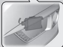
The radar sensor is in the lower bumper next to the fog light. Be careful not to have the radar sensor cover strongly impacted.
