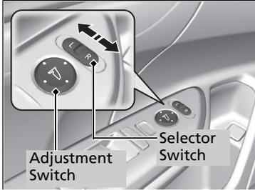
You can adjust the door mirrors when the ignition switch is in ON
