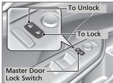
Press the master door lock switch in as shown to lock or unlock all doors.
