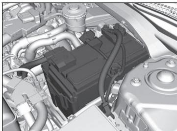
Check the battery terminals for corrosion monthly.
