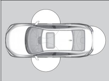
When you carry the smart entry remote, you can lock/unlock the doors, fuel fill door, and open the trunk.
