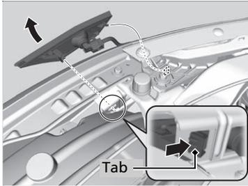
1. Push the tab to remove the light assembly.
