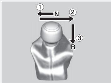
1. Depress the clutch pedal, move the shift lever all the way to the left, and shift to **N**.
