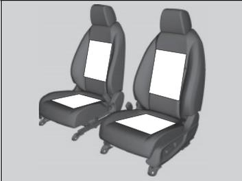
The ignition switch must be in ON **II**\*1 to use the seat heaters.
