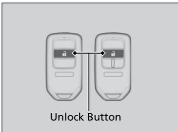
**To open:** Press the unlock button, and then within 10 seconds, press it again and hold it. If the windows and moonroof\* stop midway, repeat the procedure.
