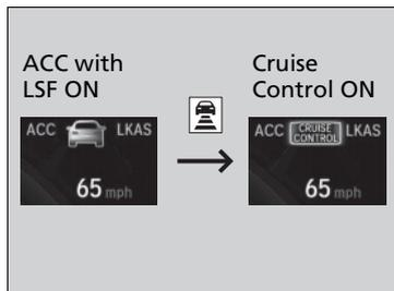
Press and hold the
