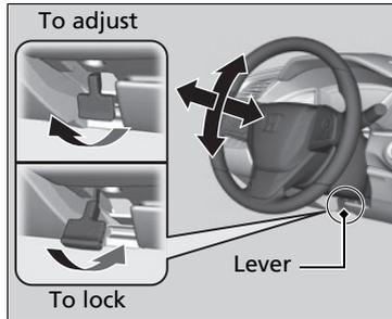
1. Pull the steering wheel adjustment lever up.
