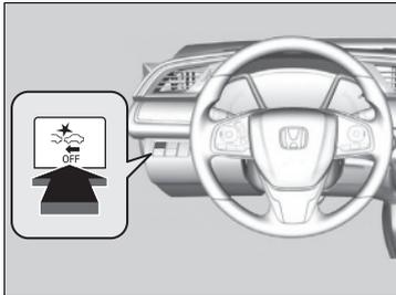
Press this button until the beeper sounds to switch the system on or off.
