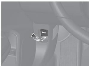
**2** Locate the hood latch lever, pull it up, and then raise the hood. Once you have raised the hood slightly, you can release the lever.
