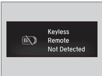
Warning buzzers may sound from inside and/or outside the vehicle to remind you that the smart entry remote is out of the vehicle. If the buzzer continues even after the remote is put back inside, place it within the system's operational range.
