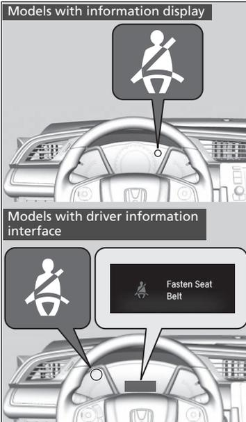
The seat belt system includes an indicator on the instrument panel to remind the driver or a front passenger or both to fasten their seat belts.
