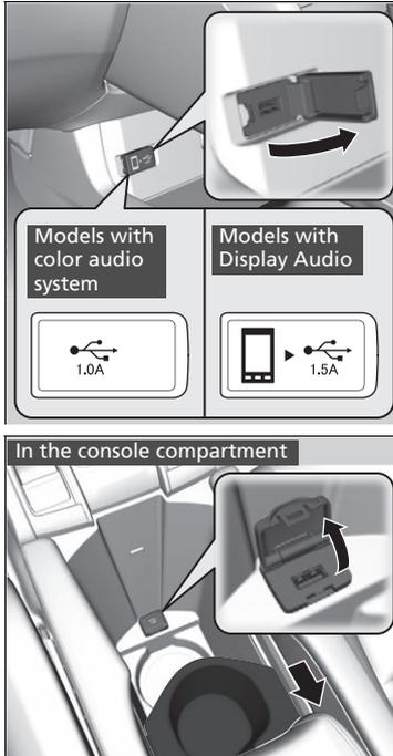
Install the iPod USB connector or the USB flash drive to the front USB port.
