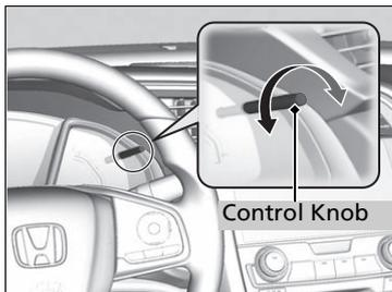
When the parking lights are turned on and the ignition switch is in ON
