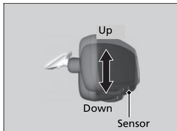
When driving after dark, the automatic dimming rearview mirror reduces the glare from headlights behind you, based in inputs from the mirror sensor. This feature is always active.
