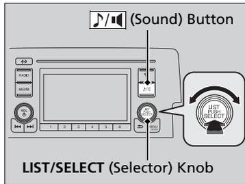
Press the (sound) button, and rotate to scroll through the following choices:
