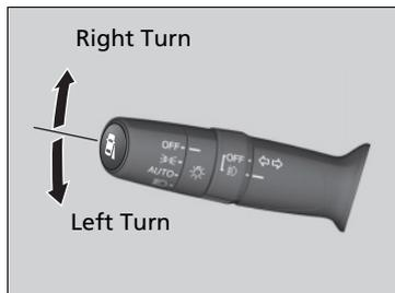
The turn signals can be used when the ignition switch is in ON
