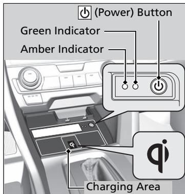
1. To turn the system on and off, press and hold the
