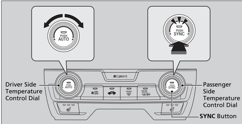
You can set the temperature synchronously for the driver's side and the passenger's side in synchronized mode.
