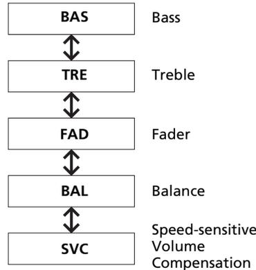
Rotate to adjust the sound setting, then press .
