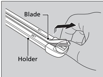
**6.** Pull the wiper blade in the opposite direction to slide it out of its holder.
