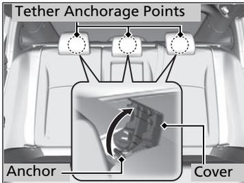
A tether anchorage point is provided behind each rear seating position. If you have a child restraint system that comes with a tether but can be installed with a seat belt, the tether may be used for additional security.
