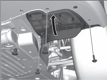
1. Remove the clips using a flat-tip screwdriver, lift and remove the bolt, and push up the under cover.
