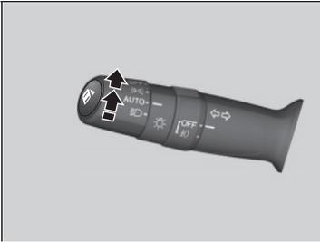
Automatic lighting control can be used when the ignition switch is in ON
