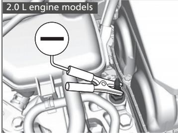
4. Connect the other end of the second jumper cable to the engine mounting bolt as shown. Do not connect this jumper cable to any other part.
