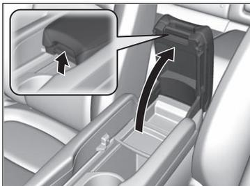
Your vehicle has a multi-function center console. It includes a storage compartment, an armrest, and a sliding tray\*. Slide the armrest to the rearmost position. Pull the handle to open the console compartment.
