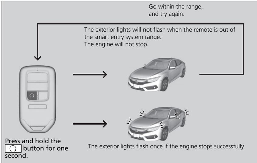
⊞ Remote Engine Start with Vehicle Feedback\*
