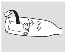
The rotating switch on the left lever controls the lights. Turning this switch to the " FOGE" position turns on the parking lights, taillights, instrument panel lights, side-marker lights, and rear license plate light. Turning the switch to the " \(\beta\)D" position turns on the headlights.
