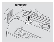
Check the engine oil level every time you fill the vehicle with fuel. Wait a few minutes after turning the engine off before you check the oil.
