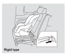
3. Put the child seat in the rear left or right vehicle seat and attach the child seat to the lower anchors according to the child seat maker's instructions.
