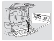
You can open the tailgate only when the hatch is open. To open the tailgate, slide the lock lever to the left and swing down the tailgate. To close the tailgate, lift it up and push it firmly until it latches.
