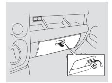
Open the glove box by pulling the bottom of the handle. Close it with a firm push. Lock or unlock the glove box with the master key.
