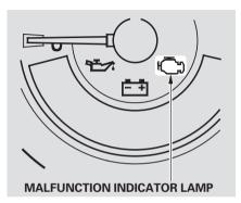
This indicator should light when the ignition switch is ON (II), and go out after the engine starts. If it comes on at any other time, it indicates one of the engine's emissions control systems may have a problem. Even though you may feel no difference in your vehicle's performance, it can reduce your fuel economy and cause vour vehicle to put out excessive emissions. Continued operation may cause serious damage.
