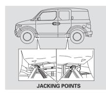
9. Locate the jacking point nearest the tire you need to change. It is pointed to by an arrow molded into the underside of the body. Place the jack under the jacking point. Turn the end bracket clockwise until the top of the jack contacts the jacking point. Make sure the jacking point tab is resting in the iack notch.
