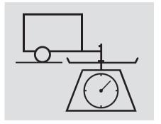
• Tongue Load: The weight that the tongue of a fully-loaded trailer puts on the hitch should be approximately 10 percent of the trailer weight. Too little tongue load can make the trailer unstable and cause it to sway. Too much tongue load reduces front-tire traction and steering control.
