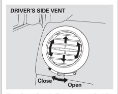
To adjust the air flow from each side vent, move the tab in the center of each vent side-to-side, and rotate the vent with the tab.
