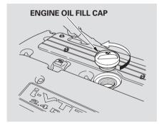
To add oil, unscrew and remove the engine oil fill cap on top of the valve cover. Pour in the oil, and install the engine oil fill cap. Tighten it securely. Wait a few minutes and recheck the oil level. Do not fill above the upper mark; you could damage the engine. Pour the oil slowly and carefully so vou do not spill. Clean up any spills immediately. Spilled oil could damage components in the engine compartment.
