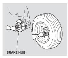
12. Before mounting the spare tire, wipe any dirt off the mounting surface of the wheel and hub with a clean cloth. Wipe the hub carefully, it may be hot from driving.
