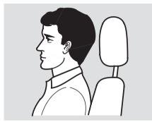
Before driving, make sure everyone with an adjustable head restraint has properly positioned the head restraint. The restraint should be positioned so the back of the occupant's head rests against the center of the restraint. A taller person should adjust the restraint as high as possible.
