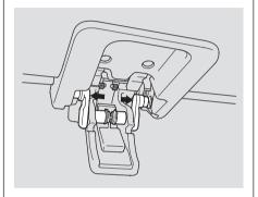
To reinstall the skylight, reverse the removal procedure, making sure the air deflector is pushed down. When reinstalling the lever assembly, align both pivots with the receptacle holes, let the pivots move out until they rest in the holes securely. Make sure the skylight is fully closed and latched.
