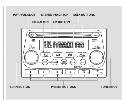
TUNE — Use the TUNE knob to tune the radio to a desired frequency. Turn the TUNE knob to the right to tune to a higher frequency, or to the left to tune to a lower frequency. Stop turning the knob when the display reaches the desired frequency.
