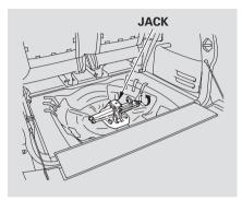
7. Remove the tools and the jack. To remove the jack, turn the jack's end bracket counterclockwise to loosen it.
