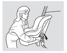
1. With the child seat in the desired seating position, route the belt through the child seat according to the seat maker's instructions, then insert the latch plate into the buckle.
