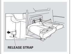
2. Pull the release strap on the seat support to unlock the seat support.
