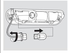
3. Pull the bulb straight out of its socket. Push the new bulb straight into the socket until it bottoms.
