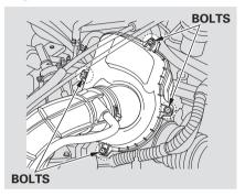
The air cleaner element is inside the air cleaner housing on the left side of the engine compartment.
