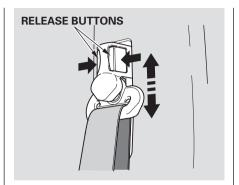
To adjust the height of a front seat belt anchor, squeeze the two release buttons and slide the anchor up or down as needed (it has four positions). Never place the shoulder portion of a lap/shoulder belt under your arm or behind your back. This could cause very serious injuries in a crash.
