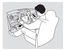
Park (P) — This position mechanically locks the transmission. Use Park whenever you are turning off or starting the engine. To shift out of Park, you must press on the brake pedal and have your foot off the accelerator pedal. Press the release button on the side of the shift lever to move it out of park.
