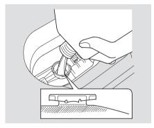
8. Pour Honda All Season Antifreeze/Coolant Type 2 into the radiator up to the base of the filler neck. This coolant is a mixture of 50 percent antifreeze and 50 percent water. Pre-mixing is not required. The cooling system capacity is:
