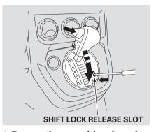
6 Remove the screwdriver from the Shift Lock Release slot, then install a new cover. Make sure the notch on the cover is on the right side. Press the brake pedal, and restart the engine.
