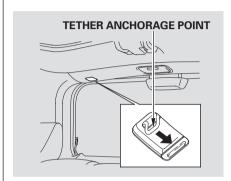
The tether anchorage points are located under plastic covers. Select the anchorage point you want to use, and slide the cover to open it.
