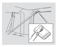
Attach the attaching clip to the tether anchorage point as shown in the illustration, then tighten the strap according to the child seat maker's instructions. Make sure the strap is not twisted.
