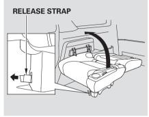
3. Pull the release strap on the seat support, and pivot the seat toward the vehicle's side wall.
