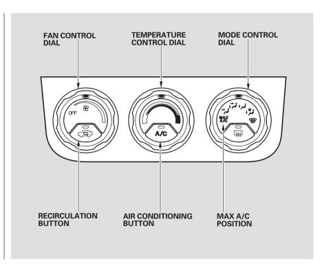
Air conditioning places an extra load on the engine. Watch the engine coolant temperature gauge (see page 74) when driving in stop-and-go traffic or climbing a long, steep hill. If it moves near the red zone, turn off the A/C until the gauge reads normally.
