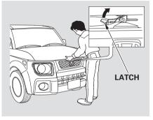
2. Standing in front of the vehicle, put your fingers between the front edge of the hood and the front grille. The hood latch handle is above the "H" logo. Push this handle up until it releases the hood. Lift the hood.
