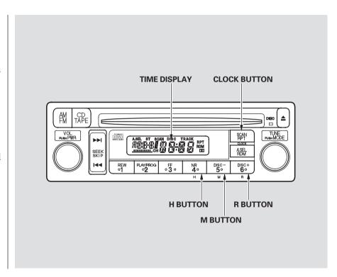
To set the hour, press the H (Preset 4) button while pressing the CLOCK (SCAN/RPT) button. Press and hold the H button until the hour advances to the desired time.
