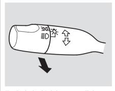
To flash the high beams, pull the turn signal lever back lightly, then release it. The high beams will come on and go off. The high beams will stay on for as long as you hold the lever back, no matter what position the headlight switch is in.
