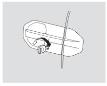
The front doors can be locked and unlocked from the outside with the key.
