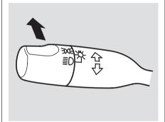
To change from low beams to high beams, push the turn signal lever forward until you hear a click. The blue high beam indicator will light (see page 69). To return to low beams, pull the turn signal lever back.
