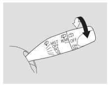
The rotating switch on the right lever controls the rear window wiper and washer.
