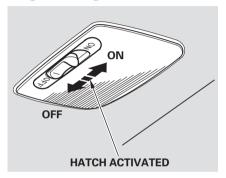
The cargo area light has a threeposition switch. In the OFF position, the light does not come on. In the center position, the light comes on when you open the hatch. In the ON position, the light stays on continuously.
