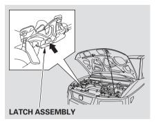
Clean the hood latch assembly with a mild cleaner, then lubricate it with a multipurpose grease. Lubricate all the moving parts (as shown), including the pivot. Follow the time and distance recommendations in the Maintenance Schedule. If you are not sure how to clean and grease the latch, contact your Honda dealer.
