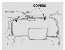
Your vehicle has two tether anchorage points on the ceiling near the hatch opening for securing a tether-style child seat to the vehicle.
