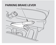
To apply the parking brake, pull the lever up fully. To release it, pull up slightly, push the button, and lower the lever. The parking brake light on the instrument panel should go out when the parking brake is fully released (see page 66).
