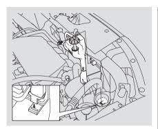
5. Remove the reserve tank mounting bolt with a wrench, and remove the reserve tank from its bottom holder by pulling it up while rotating it about 360° to avoid hitting the fan shroud.
