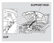
3. Pull the support rod out of its clip and insert the end into the hole in the hood
