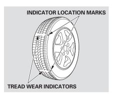
Your vehicle's tires have wear indicators molded into the tread. When the tread wears down to that point, you will see a 5/16 inch (7.9 mm) wide band running across the tread. This shows there is less than 1/16 inch (1.6 mm) of tread left on the tire. A tire that is this worn gives very little traction on wet roads. You should replace the tire if you can see the tread wear indicator in three or more places around the tire.
