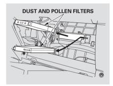
3. Remove the first filter by pulling it straight out of the air conditioning unit. Remove the second filter by sliding it to the left, then pulling it 011f.
