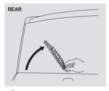
Rear: Raise the wiper arm off the hatch glass and hold it.
