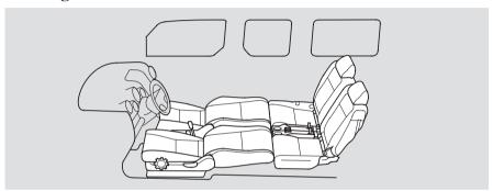
You can recline the seat-backs on the front seats to a fully flat position so they are level with the rear seat cushions, making a large cushioned area. To do this:
