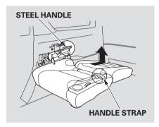
5. Hold the steel handle next to the lock lever and the holding strap at the outside edge of the seat cushion, and remove the entire seat by pulling it up and backward. Reverse this procedure to reinstall the seat. Make sure the seat is securely locked.
