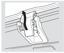
To close the skylight, pull down the lever to unlock the skylight, then push it back in place. Make sure the skylight is fully closed and locked.
