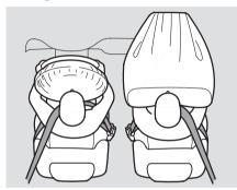
Your vehicle has a Supplemental Restraint System (SRS) with front airbags to help protect the heads and chests of the driver and a front seat passenger during a moderate to severe frontal collision.
