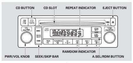
You can also play 3-inch (8-cm) discs without using an adapter ring. Play only standard round discs. Oddshaped CDs may iam in the drive or cause other problems.
