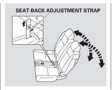
The seat-back angle of each rear seat can be adjusted separately.
