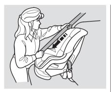
2. To activate the lockable retractor, slowly pull the shoulder part of the belt all the way out until it stops, then let the belt feed back into the retractor (you might hear a clicking noise as the belt retracts).
