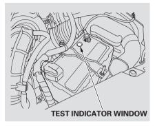
Check the battery condition by looking at the test indicator window on the battery. The label on the battery explains the test indicator's colors.
