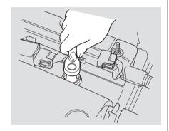
8. Torque the spark plug. (If you do not have a torque wrench, tighten the spark plug two-thirds of a turn after it contacts the cylinder head.) Tightening torque:
