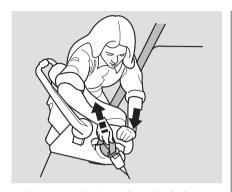
4. After confirming that the belt is locked, grab the shoulder part of the belt near the buckle and pull up to remove any slack from the lap part of the belt. Remember, if the lap part of the belt is not tight, the child seat will not be secure. To remove slack, it may help to put weight on the child seat, or push on the back of the seat, while pulling up on the belt.
