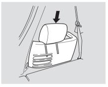
1. Remove the head restraints from the front seats (see page 94). Store the head restraints in the side pockets of the cargo area.
