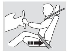
Any driver who sits too close to the steering wheel is at risk of being seriously injured or killed by striking the steering wheel or from being struck by an inflating front airbag during a crash.
