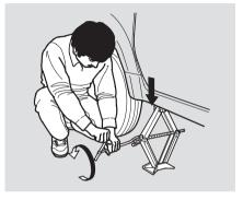
14. Lower the vehicle to the ground and remove the jack.
