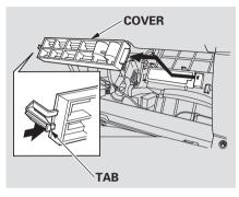
2. Remove the dust and pollen filter cover by pushing in on the lock tab, then pulling the cover toward you.
