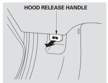
1. Shift to Park or Neutral and set. the parking brake. Pull the hood release handle located under the lower left corner of the dashboard. The hood will pop up slightly.
