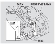
Look at the coolant level in the radiator reserve tank. Make sure it is between the MAX and MIN lines. If it is below the MIN line, see **Adding** Engine Coolant on page 225 for information on adding the proper coolant.
