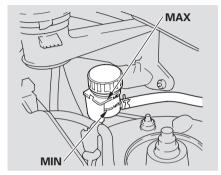
The fluid level should be between the MIN and MAX marks on the side of the reservoir. If it is not, add brake fluid to bring it up to that level. Use the same fluid specified for the brake system.
