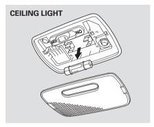
1. Remove the lens by carefully prying on the edge of the lens with a fingernail file or a small flat-tip screwdriver. Do not pry on the edge of the housing around the lens.
