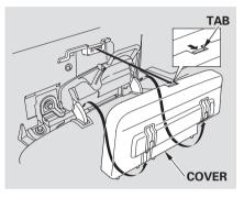
3. Remove the cover between the seat cushion and the side wall by pulling the tab and pulling the cover straight up.
