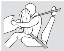
Your vehicle is equipped with dualstage, dual-threshold airbags to help reduce the chance of airbag-caused injuries.
