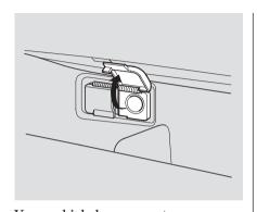
Your vehicle has one or two accessory power sockets, depending on the model. All models have a front accessory power socket on the dashboard above the glove box.
