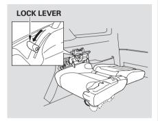
4. Push the lock lever forward to unlock the seat.
