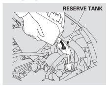
If the coolant level in the reserve tank is at or below the MIN line, add coolant to bring it up to the MAX line. Inspect the cooling system for leaks. The coolant you add should always be a mixture of 50 percent antifreeze and 50 percent water. Never add straight antifreeze or plain water.
