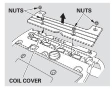
Remove the four nuts with a wrench, then remove the coil cover.
