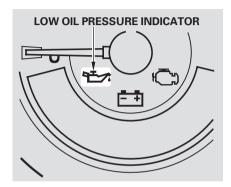
This indicator should light when the ignition switch is ON (II), and go out after the engine starts. It should never come on when the engine is running. If it starts flashing, it indicates that the oil pressure dropped very low for a moment, then recovered. If the indicator stays on with the engine running, it shows that the engine has lost oil pressure and serious engine damage is possible. In either case, you should take immediate action.
