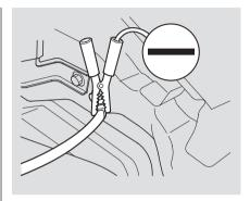
4. Connect the second jumper cable to the negative (—) terminal on the booster battery. Connect the other end to the grounding strap as shown. Do not connect this jumper cable to any other part of the engine.
