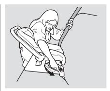
1. With the child seat in the desired back seating position, route the belt through the child seat according to the seat maker's instructions, then insert the latch plate into the buckle.
