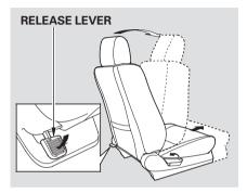
Although your vehicle has rear doors, the rear seat passengers can get out of the vehicle from the open front passenger's door. Push down on the release lever at the base of the front passenger's seat-back, and push the seat-back forward. The seat-back will tilt forward and the entire seat will move forward to allow easier exit through the front door.
