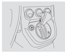
Push the button next to the shift lever to turn on the hazard warning lights (four-way flashers). This causes all four outside turn signals and both indicators in the instrument panel to flash. Use the hazard warning lights if you need to park in a dangerous area near heavy traffic, or if your vehicle is disabled.
