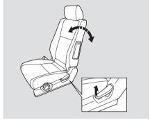
To change the angle of the seat-back, pull up on the lever on the outside of the seat bottom. Move the seat-back to the desired position and release the lever. Let the seat-back latch into the new position.
