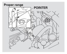
An auto-tensioner adjusts the tension of the drive belt. The pointer on the auto-tensioner should be in the proper range. It should be checked according to the time and distance recommendations in the maintenance schedule.
