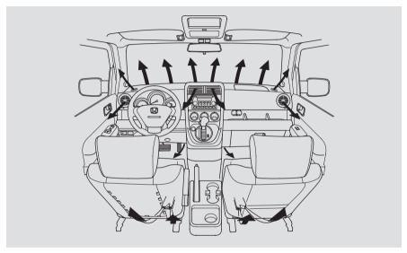
EX models When you select if or if the system automatically switches to Fresh Air mode and turns on the A/C.
