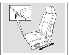
To adjust the seat forward and backward, pull up on the bar under the seat cushion's front edge. Move the seat to the desired position and release the bar. Try to move the seat to make sure it is locked in position.
