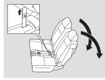
4. Adjust the rear seat-back to the desired position.
