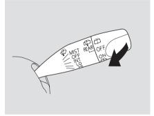
To clean the windshield, pull back on the wiper control lever. The washers spray until you release the lever. The wipers run at low speed while you're pulling the lever, then complete one more sweep of the windshield after you release it.
