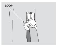
If your seat belts get dirty, you can use a soft brush with a mixture of mild soap and warm water to clean them. Do not use bleach, dye, or cleaning solvents. They can weaken the belt material. Let the belts airdry before you use the vehicle.
