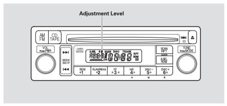
**Treble/Bass** — Use these modes to adjust the tone to your liking. Select TRE or BAS by pressing the TUNE knob. Adjust the desired mode by turning the TUNE knob. The displayed number shows you the current setting. When the adjustment level reaches the center, you will see "  $\mathcal{L}$  ".
