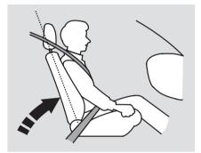
Adjust the driver's seat-back to a comfortable, upright position, leaving ample space between your chest and the airbag cover in the center of the steering wheel. If you sit too close to the steering wheel, you could be injured if the front airbag inflates.
