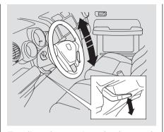
To adjust the steering wheel upward or downward:
