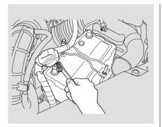
If the terminals are severely corroded, clean them with baking soda and water. Then use a wrench to loosen and remove the cables from the terminals. Always disconnect the negative (—) cable first and reconnect it last. Clean the battery terminals with a terminal cleaning tool or wire brush. Reconnect and tighten the cables, then coat the terminals with grease.
