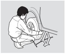
11. Remove the wheel nuts and flat tire. Temporarily place the flat tire on the ground with the outside surface of the wheel facing up. Placing the wheel face down could mar its finish.
