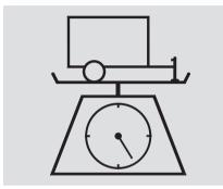
• Total Trailer Weight: The total weight of the trailer and everything loaded in it must not exceed 1,500 lbs (680 kg). Towing a load that is too heavy can seriously affect your vehicle's handling and performance. It can also damage the engine and drivetrain.
