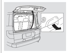
With the hatch unlocked, open it by pulling the handle and lifting up. To close the hatch, lower it, then press down on the back edge.
