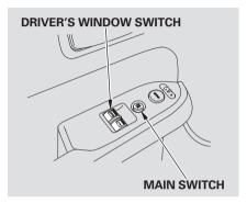
The driver's door armrest has a master power window control panel. To open the passenger's window, push down on the switch and hold it until the window reaches the desired position. To close the window, pull back on the window switch. Release the switch when the window gets to the position you want.
