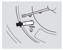
Push the knob in the speedometer repeatedly to adjust the brightness of the instrument panel lights. There are six brightness levels. A segment display shows the current brightness level.
