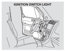
The ignition switch light comes on when you unlock the driver's door, and fades out about 30 seconds after you close the door.
