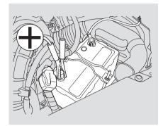
3. Connect one jumper cable to the positive (+) terminal on your Honda's battery. Connect the other end to the positive (+) terminal on the booster battery.
