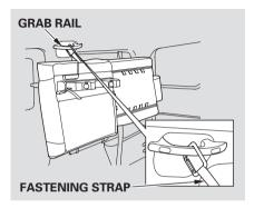
4. A fastening strap is attached to the inside of the seat cushion. While pushing the seat up and toward the side wall, hook the fastening strap to the grab rail.
