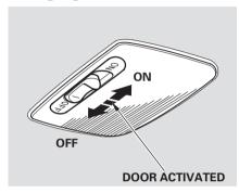
The ceiling light has a three-position switch. In the OFF position, the light does not come on. In the center position, the ceiling light comes on when you open any door. After all doors are closed tightly, the light fades out in about 30 seconds. In the ON position, the ceiling light stays on continuously.
