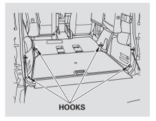
To secure cargo, use the four cargo hooks in the cargo area floor. There is another hook on each side wall near the hatch. Make sure all stored items are secured before driving.
