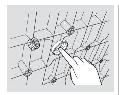
19. Remove the small round plug from the cargo area floor by pushing it from the back side to make a hole. Store the removed plug in a place you can easily remember.
