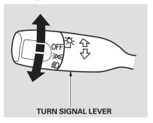
Signal a turn or lane change with this lever. Push down on the lever to signal a left turn, and up to signal a right turn. If you push it up or down all the way, the turn signal continues to blink even when you release the lever. It shuts off automatically as you complete the turn.
