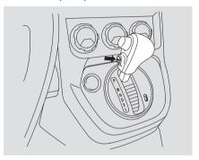
Overdrive (O/D) is on whenever you turn the ignition ON (II). You can turn it off by pressing the O/D switch on the end of the shift lever. The O/D OFF indicator on the instrument panel next to the shift lever "D" position indicator will come on.
