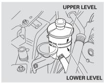
Check the level when the engine is cold. Look at the side of the reservoir. The fluid should be between the UPPER LEVEL and LOWER LEVEL. If it is below the LOWER LEVEL, add power steering fluid to the UPPER LEVEL.
