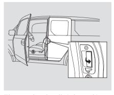
The rear door handle is located in the rear door edge. The rear door can be opened only when the front door is open. Pull the handle to open the rear door.
