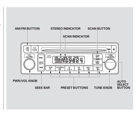
You can use any of five methods to find radio stations on the selected band: TUNE, SEEK, SCAN, AUTO SELECT, and the preset buttons.
