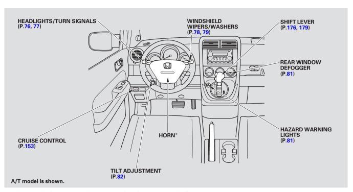
$\boldsymbol{\ast}$  : To use the horn, press the center pad of the steering wheel.
