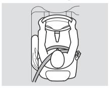
Optional on EX model Your vehicle is equipped with side airbags for the driver and a front seat passenger. The airbags are stored in the outer edges of the front seat-backs, and both are marked "SIDE AIRBAG."
