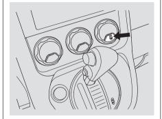
The rear window defogger will clear fog, frost, and thin ice from the window. Push the defogger button to turn it on and off. The light in the button lights to show the defogger is on.
