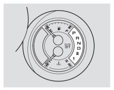
This indicator on the instrument panel shows which position the shift lever is in. The "D" indicator comes on for a few seconds when you turn the ignition switch to ON (II). If it flashes while driving (in any shift position), it indicates a possible problem in the transmission. Avoid rapid acceleration and have the transmission checked by an authorized Honda dealer as soon as possible.
