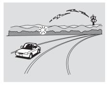
Driving very near the transmitter of a station that is broadcasting on a frequency close to the frequency of the station you are listening to can also affect your radio's reception. You may temporarily hear both stations, or hear only the station you are close to.
