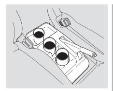
The center console has three beverage holders for the front and rear passengers.
