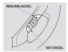
3. Press and release the SET/ DECEL button on the steering wheel The CRUISE CONTROL light on the instrument panel comes on to show the system is now activated.
