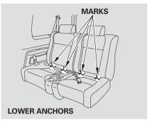
Your vehicle is equipped with LATCH (Lower Anchors and Tethers for Children) at the rear seats. The lower anchors are located between the seat-back and seat bottom and are to be used only with a child seat designed for use with LATCH.
