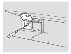
An auxiliary input jack is located on the dashboard next to the accessory power socket. Your audio system will accept auxiliary inputs from a portable cassette player, CD changer, MP3 player, etc. To use the jack, turn down the volume of the audio unit and the portable unit. Then pivot the cover up, plug in a mini-jack cable between the portable unit and the jack, and press the AUX button on the audio unit.
