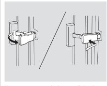
To open a rear window, pull the lever towards you, then push it out until it locks. To close the rear window pull the lever towards you, then push it back. Make sure the window is fully closed and locked.
