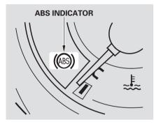
The ABS is self-checking. If anything goes wrong, the ABS indicator on the instrument panel comes on (see page 68). This means the anti-lock function of the braking system has shut down. The brakes still work like a conventional system without anti-lock, providing normal stopping ability. You should have the dealer inspect your vehicle as soon as possible.
