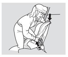
4. After confirming that the belt is locked, grab the shoulder part of the belt near the buckle and pull up to remove any slack from the lap part of the belt. Remember, if the lap part of the belt is not tight, the child seat will not be secure. It may help to put weight on the child seat, or push on the back of the seat, while pulling up on the belt.
