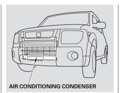
Run the air conditioning at least once a week during the cold weather months. Run it for at least ten minutes while you are driving at a steady speed with the engine at normal operating temperature. This circulates the lubricating oil contained in the refrigerant.
