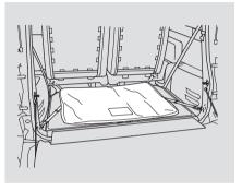
With the rear seats in their upright position, store the skylight, face down in its bag in the cargo area. Secure the bag with four hooks on the cargo area floor. Do not store anything on top of the skylight.
