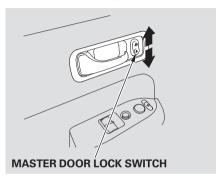
The master door lock switch on the driver's door locks and unlocks all of the doors and the hatch. Push the switch down to lock all of the doors and the hatch, and up to unlock them.
