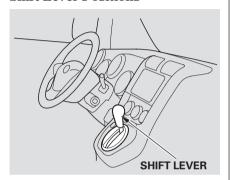
The shift lever has six positions. It must be in Park or Neutral to start the engine. When you are stopped in D, 2, 1, N, or R, press firmly on the brake pedal, and keep your foot off the accelerator pedal.
