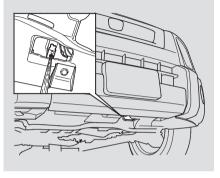
4. Loosen the drain plug on the bottom of the radiator. The coolant will drain through the splash guard.
