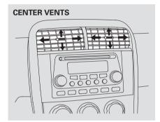
The direction of air flow from the vents in the center and each side of the dashboard is adjustable.
