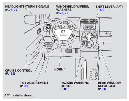
\*: To use the horn, press the center pad of the steering wheel.
