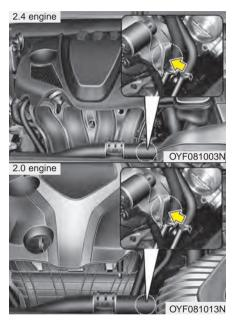
The engine number is stamped on the engine block as shown in the drawing.
