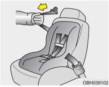
Pull the shoulder portion of the seat belt all the way out. When the shoulder portion of the seat belt is fully extended, it will shift the retractor to the "Aautomatic locking" (child restraint) mode.
