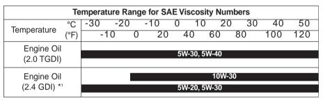
\*1. For better fuel economy, it is recommended to use the engine oil of a viscosity grade SAE 5W-20 (API SM / ILSAC GF-4). However, if the engine oil is not available in your country, select the proper engine oil using the engine oil viscosity chart.
