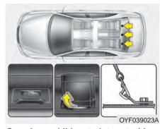
Securing a child restraint seat with "Tether Anchor" system
