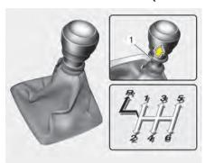
The shift lever can be moved into any of the forward gears without pulling the ring (1).
