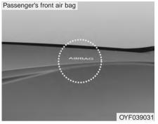
The purpose of the SRS is to provide the vehicle's driver and/or the front passenger with additional protection than that offered by the seat belt system alone in case of a frontal impact of sufficient severity. The SRS uses sensors to gather information about the driver's seat position, the driver's and front passenger's seat belt usage and impact severity.
