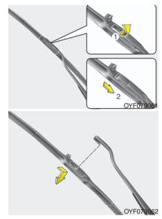
Lift up the wiper blade clip. Then pull down the blade assembly and remove it.
