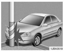
Air bags may not inflate if the vehicle collides with objects such as utility poles or trees, where the point of impact is concentrated to one area and the deceleration forces are significantly reduced.
