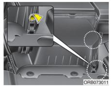
1. Loosen the air cleaner cover attaching clips and open the cover.
