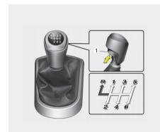
The shift lever can be moved into any of the forward gears without pressing the button (1).
