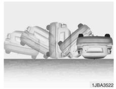
Front air bags do not inflate in rollover accidents. However, side impact and curtain air bags may inflate in a rollover, when it is detected by the rollover sensor.
