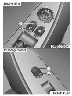
With central door lock switch (if equipped)
