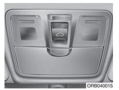
If your vehicle is equipped with a sunroof, you can slide or tilt your sunroof with the sunroof control switch located on the overhead console
