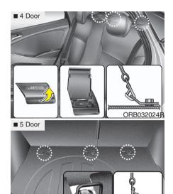
Securing a child restraint seat with "Tether Anchor" system
