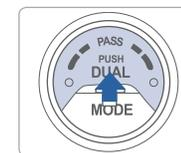
Press the DUAL button to operate the driver's and passenger's side temperature individually.
