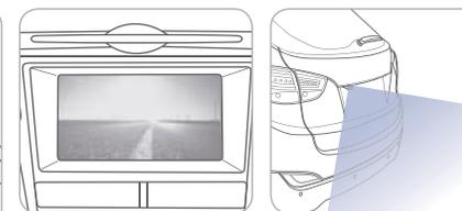
The rearview camera will activate when the ignition switch is ON and the shift lever is in the R (Reverse) position.
