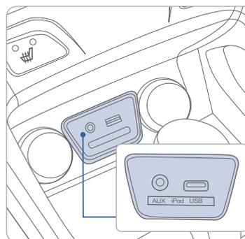
Use the jack to connect an external audio device and listen to it through the audio system in your vehicle.
