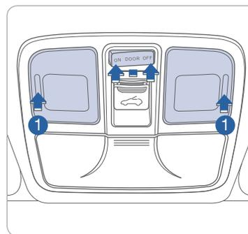
Press the lens ① to turn the map lamp on or off.
