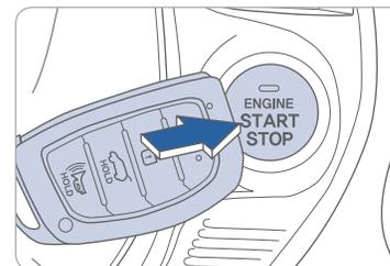
If the smart key battery is weak or the smart key does not work correctly, press the Engine Start/Stop button with the smart key in the direction of the picture.
