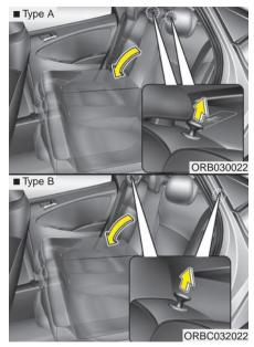
Pull on the seatback folding lever, then fold the seat toward the front of the vehicle.
