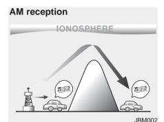
AM broadcasts can be received at greater distances than FM broadcasts. This is because AM radio waves are transmitted at low frequencies. These long distance, low frequency radio waves can follow the curvature of the earth rather than travelling straight. In addition, they curve around obstructions resulting in better signal coverage.
