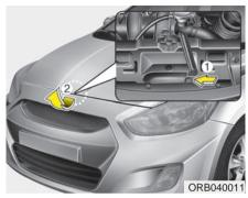
2. Go to the front of the vehicle, raise the hood slightly, push the secondary latch (1) to the left and lift the hood (2).
