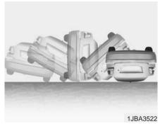
Front air bags may not inflate in rollover accidents because air bag deployment would not provide additional protection to the occupants.
