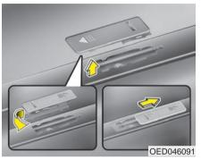
Rotate the cover half way and insert the cover on the roof hole as the illustration
