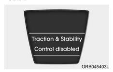
Press the ESC OFF button for more than 3 seconds. ESC OFF indicator light and message illuminates and ESC OFF warning chime will sound. At this state, the engine control function and brake control function does not operate. In other words, the vehicle stability control function does not operate any more.
