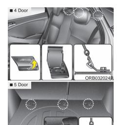
Securing a child restraint seat with "Tether Anchor" system
