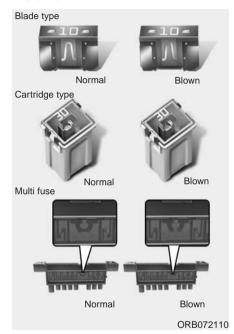
A vehicle's electrical system is protected from electrical overload damage by fuses. This vehicle has 2 fuse panels, one located in the driver's side panel bolster, the other in the engine compartment.
