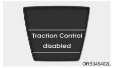
Press the ESC OFF button shortly (ESC OFF indicator light and message illuminates). At this state, the engine control function does not operate. In other words, the traction control function does not operate but only the brake control function operates.
