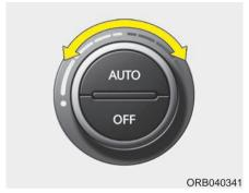
2. Turn the temperature control knob to set the desired temperature.
