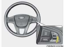
3. Move the toggle switch down (to SET-), and release it at the desired speed. The SET indicator light in the instrument cluster will illuminate. Release the accelerator at the same time. The desired speed will automatically be maintained.
