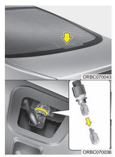
High mounted stop light bulb replacement (if equipped)
