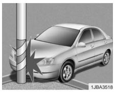
Air bags may not inflate if the vehicle collides with objects such as utility poles or trees, where the point of impact is concentrated to one area and the deceleration forces are significantly reduced.
