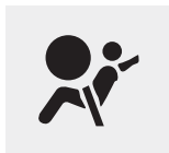
SRS warning light
