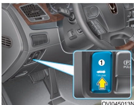
(1) Power Trunk Main Control button
