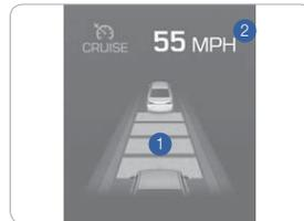
If your vehicle is equipped with Advanced Smart Cruise Control and you wish to eliminate the vehicle distance function, you can change cruise control setting to a standard setting.
