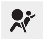
SRS warning light
