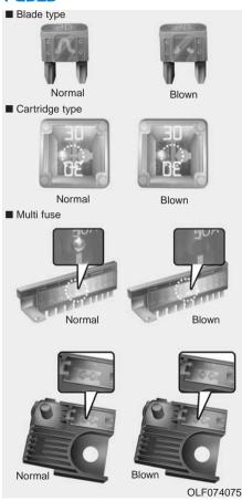
A vehicle's electrical system is protected from electrical overload damage by fuses.
