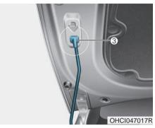
4. Pull out the support rod and hold the hood open with the support rod (3).
