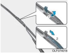
2. Lift the wiper blade clip. Then push down the blade body.
