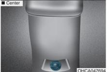
The power outlet is designed to provide power for mobile telephones or other devices designed to operate with vehicle electrical systems. The devices should draw less than 180 W (Watts) with the engine running.
