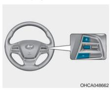
The LCD display modes can be changed by using the control buttons.
