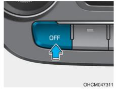
Push the OFF button to turn the climate control system off. You can still operate the mode and air intake buttons as long as the ignition switch is in the ON position.
