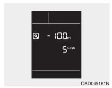
To reset the service interval, press the RESET button for more than 5 seconds and then when the miles and days blink press the RESET button for more than 1 second.
