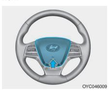
To sound the horn, press the area indicated by the horn symbol on your steering wheel (see illustration). The horn will operate only when this area is pressed.
