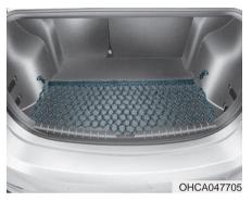
To keep items from shifting in the luggage compartment, you can use the 4 holders located in the luggage compartment to attach the luggage net.
