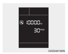
If the remaining mileage or time reaches 900 miles (1,500 km) or 30 days, the service symbol ( ) will blink for several seconds each time you set the ignition switch or Engine Start/Stop button to the ON position.
