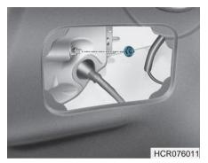
3. Loosen the lamp assembly retaining screws with a cross-tip screwdriver.
