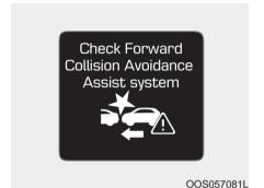
Check Forward Collision Avoidance Assist system
