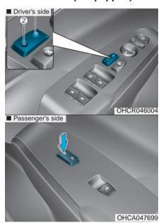
When pressing the  $( \frac{}{\Box} )$  switch (1), all vehicle doors will lock.
