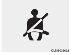
As a reminder to the driver, the seat belt warning light will illuminate for approximately 6 seconds each time you place the ignition switch to the ON position regardless of belt fastening. However, if the seat belt is unfasted, a warning chime will sound for approximately 6 seconds.
