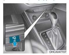
When the ignition switch is in the ON position or when the engine is running, press the heated steering wheel button to warm the steering wheel. The indicator on the button will illuminate.
