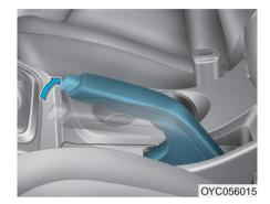
Always set the parking brake before leaving the vehicle. To apply the parking brake:
