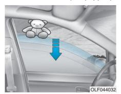
If a window senses any obstacle while it is closing automatically, it will stop and lower approximately 12 inches (30 cm) to allow the object to be cleared.
