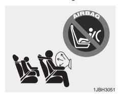
Even though your vehicle is equipped with the OCS, never install a child restraint in the front passenger's seat. An inflating air bag can forcefully strike a child or child restraint resulting in serious or fatal injury.
