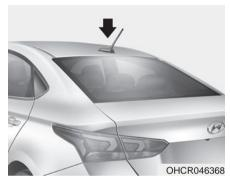
The roof antenna receives AM/FM signals.
