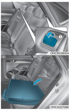
4. Pull up the seatback folding lever (1), then fold the seat toward the front of the vehicle.
