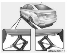
7. Place the jack at the designated jacking position under the frame closest to the tire you are changing. The jacking positions are plates welded to the frame with two notches. Never jack at any other position or part of the vehicle. Doing so may damage the side seal molding or other parts of the vehicle.
