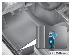
The fuel filler door must be opened from inside the vehicle by pulling the fuel filler door opener lever.
