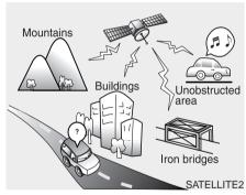
The signal can become weak in some areas that are not covered by the XM<sup>™</sup> repeater network.
