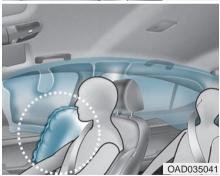
Your vehicle is equipped with a side air bag in each front seat.
