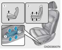
Seat cushion tilt (1, if equipped) To change the angle of the front part of the seat cushion:
