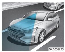
In order for the FCA system to operate properly, always make sure the camera is clean and free of dirt, snow, and debris.
