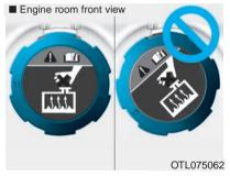
1. Check if the coolant cap label is straight In front.
