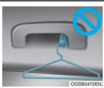
Do not hang other objects such as hangers or hard objects except clothes. Also, do not put heavy, sharp or breakable objects in the clothes pockets. In an accident or when the curtain air bag is inflated, it may cause vehicle damage or personal injury.
