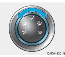
The mode selection knob controls the direction of the air flow through the ventilation system.
