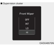
This indicator displays which wiper speed is selected using the wiper control.
