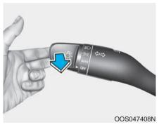
To flash the high beam headlamp, pull the lever towards you, then release the lever. The high beams will remain ON as long as you hold the lever towards you.
