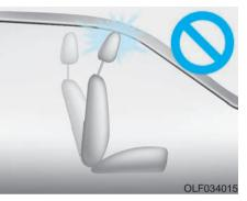
If you recline the seatback towards the front with the head restraint and seat cushion raised, the head restraint may come in contact with the sunvisor or other parts of the vehicle.
