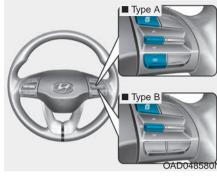
To change the trip mode, toggle the UP/DOWN arrow switch " $\blacktriangle$ ,  $\blacktriangledown$ " on the steering wheel.
