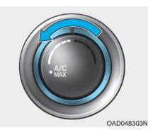
The MAX A/C mode is used to cool the inside of the vehicle faster. Air flow is directed toward the upper body and face.
