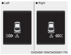
If the vehicle detected by the sensors approaches from the rear left/right side of your vehicle, the warning chime will sound, the warning light on the outside rearview mirror will blink and a message will appear on the LCD display. If the rear view monitor system is in activation, a message will also appear on the audio or AVN screen. The warning will stop when:
