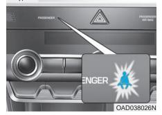
As a reminder to the front passenger, the front passenger's seat belt warning lights will illuminate for approximately 6 seconds each time you turn the ignition switch ON regardless of belt fastening.
