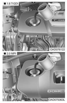
Checking the Engine Oil and Filter
