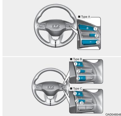
The LCD display modes can be changed by using the control buttons on the steering wheel.
