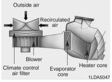
This filter is installed behind the glove box. It filters the dust or other pollutants that enter the vehicle through the heating and air conditioning system.
