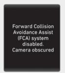
However, the FCA may not properly operate in an area (e.g. open terrain), where any substances are not detected or the camera is blocked with dirt, snow or debris after turning ON the engine.
