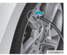
Unscrew the valve cap from the valve of the flat tire and screw the filling hose (2) of the sealant bottle onto the valve.
