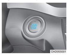
Whenever the front door is opened, the Engine Start/Stop button will illuminate and will go off 30 seconds after the door is closed.
