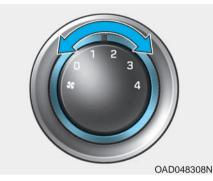
Turn the knob to the right to increase the fan speed and airflow. Turn the knob to the left to decrease fan speed and airflow.
