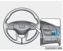
Push the toggle switch up (RES+). If the vehicle speed is over 20 mph (30 km/h), the vehicle will resume the preset speed.
