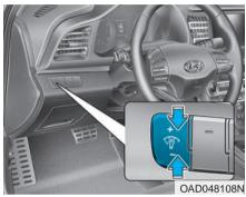
When the vehicle's parking lights or headlights are on, press the illumination control button to adjust the brightness of the instrument panel illumination.
