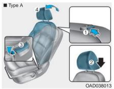
To reinstall the head restraint:
