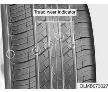
If the tire is worn evenly, a tread wear indicator will appear as a solid band across the tread. This shows there is less than 2/32 inch (1.6 mm) of tread left on the tire. Replace the tire when this happens.
