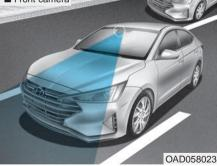
In order for the FCA system to operate properly, always make sure the sensor cover or sensor is clean and free of dirt, snow, and debris. Dirt, snow, or foreign substances on the sensor cover or sensor may adversely affect the sensing performance of the sensor.
