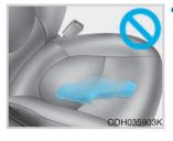
If large quantity of liquid has been spilled on the passenger seat, the air bag warning light may illuminate or malfunction.
