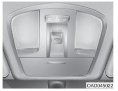
If your vehicle is equipped with a sunroof, you can slide or tilt your sunroof with the sunroof control switch located on the overhead console.
