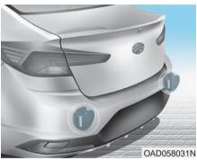
The rear radars are the sensors inside the rear bumper for detecting the side and rear areas. Always keep the rear bumper clean for proper operation of the system.
