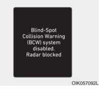
Blind-Spot Collision Warning (BCW) system disabled. Radar blocked
