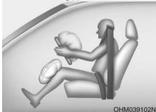
When the SRSCM detects a sufficiently severe impact to the front of the vehicle, it will automatically deploy the front air bags.
