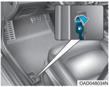
The fuel filler door must be opened from inside the vehicle by pulling up the fuel filler door release lever.
