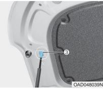
4. Pull out the support rod and prop the hood open with the support rod (3).
