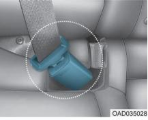
When using the rear center seat belt, the buckle with the "CENTER" mark must be used.
