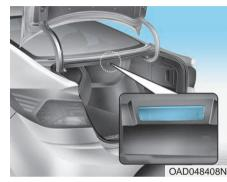
The trunk room lamp comes on when the trunk is opened.
