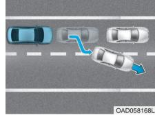
When driving in stop-and-go traffic, and a stopped vehicle in front of you merges out of the lane, the FCA system may not immediately detect the new vehicle that is now in front of you. In this case, you must maintain a safe braking distance, and if necessary, depress the brake pedal to reduce your driving speed in order to maintain a safe distance.
