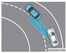
The system may not operate properly when driving on a curved road. In certain instances, the system may recognize a vehicle in the same lane.
