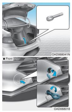
1. Open the trunk, and remove the towing hook from the tool case.
