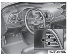
The instrument panel vent air flow can be directed up/down or left/right using the vent adjustment lever.
