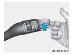
In the OFF position, pull the lever gently toward you to spray washer fluid on the windshield and to run the wipers 1-3 cycles. The spray and wiper operation will continue until you release the lever. If the washer does not work, you may need to add washer fluid to the washer fluid reservoir.
