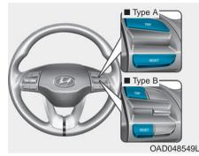
To change the trip mode, press the TRIP button on the steering wheel.
