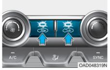
This button is used to select the outside (fresh) air position or recirculated air position.
