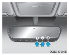
3. Press and release the programed HomeLink button to activate the garage door. 4. Once the garage door is stopped, press and release the "Learn" or "Smart" button on the Garage door opener within 1 minute from the time of pressing the programed
