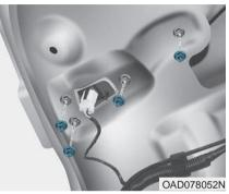
3. Disconnect the connector and then remove the nuts by turning the nuts counter clockwise.
