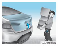
On a vehicle equipped with a smart key, the trunk can be opened using the Smart Trunk system.
