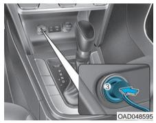
6. Plug the compressor power cord (3) into the vehicle power outlet.
