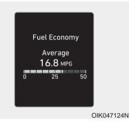
The trip computer mode displays information related to vehicle driving parameters including range, fuel economy, trip meter information and vehicle speed.
