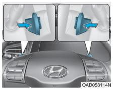
The paddle shifter is available when the shift lever is in the D (Drive) position or the manual shift mode. With the shift lever in the D position
