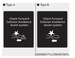
Check Forward Collision Avoidance Assist system
