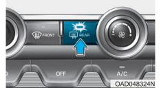
The defroster heats the window to remove frost, fog and thin ice from the interior and exterior of the rear window, while engine is running.
