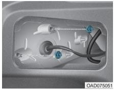
3. Loosen the assembly retaining nuts.
