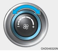
The fan speed can be set to the desired speed by turning the fan speed control knob.
