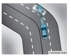
The FCA system may recognize a vehicle in the next lane when driving on a curved road.
