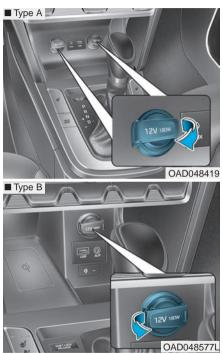
The power outlet is designed to provide power for mobile telephones or other devices designed to operate with vehicle electrical systems. The devices should draw less than 180 W (Watts) with the engine running.
