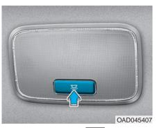
Rear Room Lamp (  $\overline{\gamma}$ ): Press this switch to turn the room lamp on and off.
