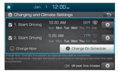
You can set the date and time of when to charge the battery and the climate control temperature. Two separate schedules can be set.
