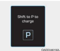
This message is displayed if you connect the charging cable without the gear in the P (Park) position.
