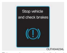
This warning message is displayed when a failure occurs in the brake system.
