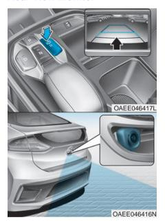
The Rear View Monitor will activate when the vehicle is in the ready () mode and when you shift to the R (Reverse) position.
