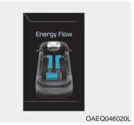
Only the motor power is used to drive the vehicle.
