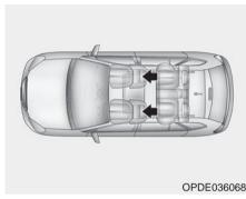
The vehicle's front and passenger's seats are equipped with adjustable head restraints for the passengers safety and comfort.
