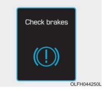
This warning message is displayed when the brake performance is low or the regenerative brake does not work properly due to a failure in the brake system.
