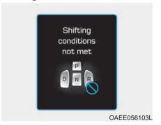
The message appears on the LCD display when driving speed is too fast to shift the gear.
