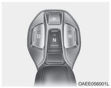
Select gear positions by pressing the shift button.
