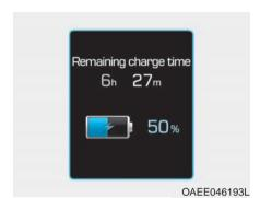
After charging has started, the estimated charging time is displayed on the instrument cluster for about 1 minute.
