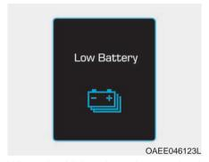
When the high voltage battery level reaches below 13%, this warning message is displayed.
