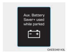
This message is displayed when the Aux. Battery Saver+ function has been operated while the vehicle was turned off.
