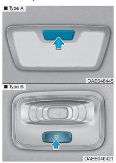
Rear Room Lamp ( $\nearrow \hookrightarrow$ ): Press this switch to turn the room lamp on and off.
