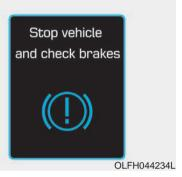
This warning message is displayed when a failure occurs in the brake system.
