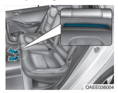
The high voltage battery cooling duct is located in the bottom center of the rear seats. The cooling duct cools down the high voltage battery.
