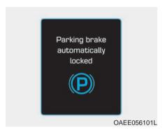
Parking brake automatically locked If the EPB is applied while Auto Hold is activated, a warning will sound and a message will appear.
