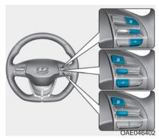
To change the trip mode, toggle the UP/DOWN arrow switch "  $\wedge$  ,  $\vee$  " on the steering wheel.
