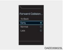
The driver can select the initial warning activation time on the LCD display. Go to the 'User Settings → Driver Assistance → Forward Collision Warning → Early/Noramal/Late'.
