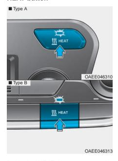
Push the HEAT button to turn the heater on (indicator light will illuminate).
