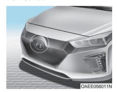
In order for the FCA system to operate properly, always make sure the radar sensor cover is clean and free of dirt, snow, and debris. Dirt, snow, or foreign substances on the lens may adversely affect the sensing performance of the sensor.
