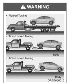
If towing is required, lift all four wheels off the ground and tow the vehicle. If you must tow the vehicle using only two wheels, lift the front wheels off the ground and tow the vehicle
