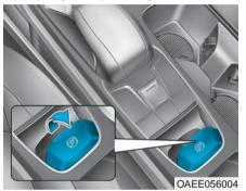
To apply the EPB (Electronic Parking Brake):
