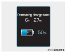
This message is displayed to notify the remaining time to fully charge the battery.
