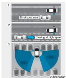
The Blind-spot Collision Warning (BCW) system uses radar sensors in the rear bumper to monitor and warn the driver of an approaching vehicle in the driver's blind spot area.
