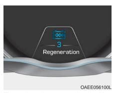
The selected regenerative braking rate is displayed on the instrument cluster.
