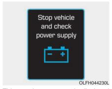
This warning message is displayed when a failure occurs in the power supply system.
