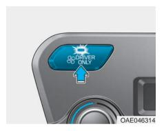
If you press the DRIVER ONLY button(\$\mathbf{s}^{\text{DRIVER}}\) and the indicator light illuminates, cold air mostly blows in the direction of the driver's seat. However, some of the cold air may come out of other seating position ducts to keep indoor air pleasant.
