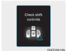
The message appears on the LCD display when there is problem with the shift buttons.
