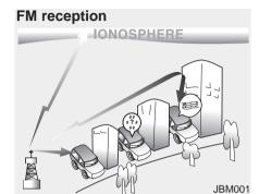
AM and FM radio signals are broadcasted from transmitter towers located around your city. They are intercepted by the radio antenna on your vehicle. This signal is then processed by the radio and sent to your vehicle speakers.
