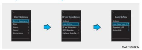
The driver can change LKA to Lane Departure Warning (LDW) System or change the LKA system mode between Active LKA and Standard LKA from the User Settings Mode on the LCD display.
