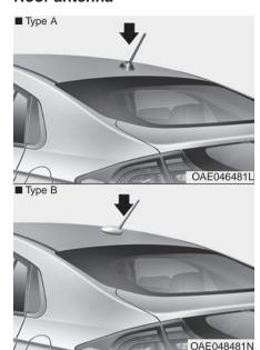
The roof antenna receives both AM and FM broadcast signals, SXM signals (only type B). Rotate the roof antenna in a counterclockwise direction to remove it. Rotate it in a clockwise direction to reinstall it.
