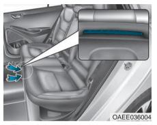
The high voltage battery cooling duct is located in the bottom center of the rear seats. The cooling duct cools down the high voltage battery. When the high voltage battery cooling duct is blocked, the high voltage battery may be overheated. Do not obstruct the cooling duct with any other objects.
