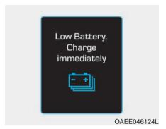
When the high voltage battery level reaches below 4%, this warning message is displayed.
